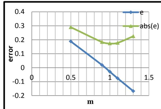
Figure 6. Variation of error and error absolute for calculating deflection if consider  $I = \left(m \frac{M_{cr}}{M_a}\right)^3 I_g + \left[1 - \left(m \frac{M_{cr}}{M_a}\right)^3\right] I_{cr}$  with change of m
