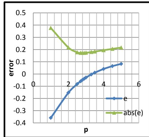
Figure 7. Variation of error and error absolute for calculating deflection if consider  $I=(\frac{M_{cr}}{M_a})^p I_g + [1 - (\frac{M_{cr}}{M_a})^p] I_{cr}$  with change of p
