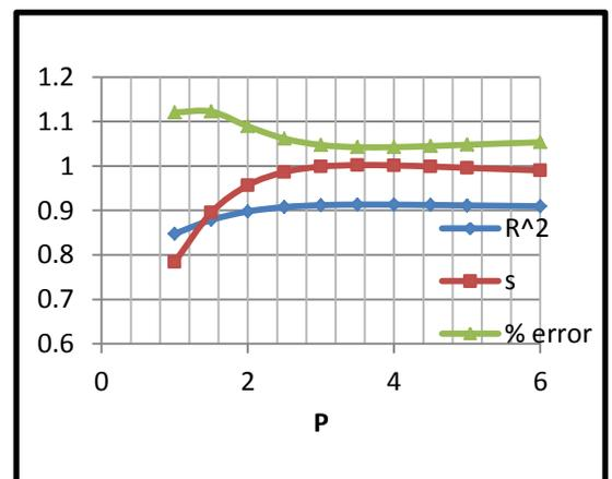
Figure 8. Variation of slope (s) of trend line and data correlation ( $R^2$ ) and % error with power (p)
