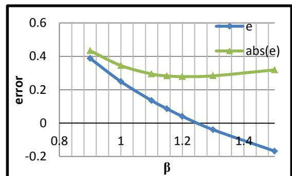
Figure 3. Variation of error and absolute error for calculating deflection if consider  $I = \beta I_{cr}$  with change of  $\beta$
