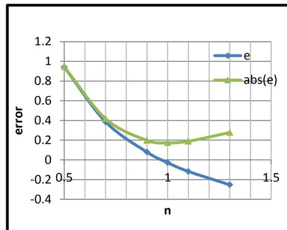
Figure 5. Variation of error and error absolute for calculating deflection if consider  $I = n I_e$  with change of n
