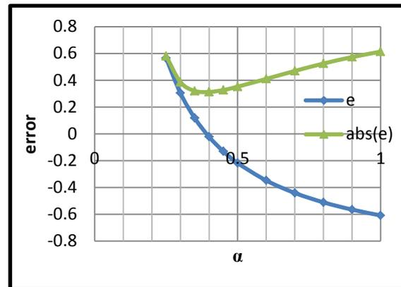
Figure 2. Variation of error and absolute error for calculating deflection if consider  $I = \alpha I_g$  with change of  $\alpha$
