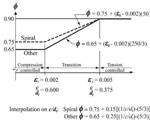
Figure 1. Variation of  $\phi$  with Tensile Strain in Rebar for Grade 60 Steel (ACI 318-11).
