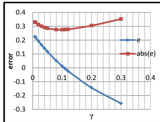
Figure 4. Variation of error and error absolute for calculating deflection if consider  $I = \gamma I_g + (1 - \gamma) I_{cr}$  with change of  $\gamma$
