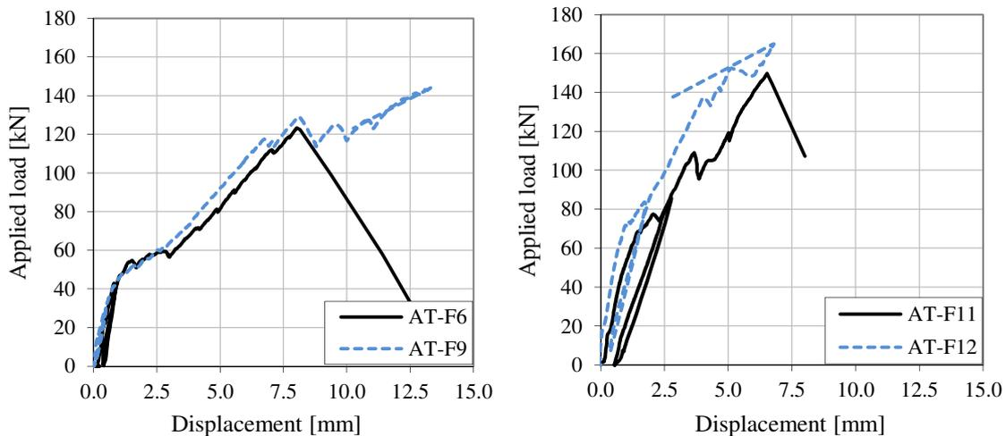
Figures 6a and b: Load-displacement curve of Series F (left: C-Sheet 200 g/m<sup>2</sup>, right: C-Sheet 400 g/m<sup>2</sup>)
