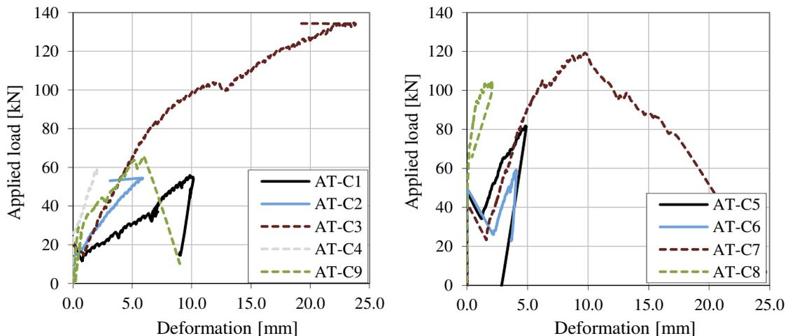
Figures 4a and 4b: Load-displacement curve of Series C (left: RHS profiles, right: L-profiles)
