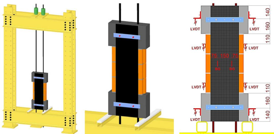
Figures 2a to 2c: Overview of test set-up (left); Detail of test set-up in Series F (middle); Measurements in Series F with SG = strain gauge and LVDT = Linear variable differential transformer (right)
