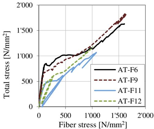
Figure 7: Comparison of measured fiber stress (strain gauges) and total stress ( $F/A_{Fiber}$ ) in Series F
