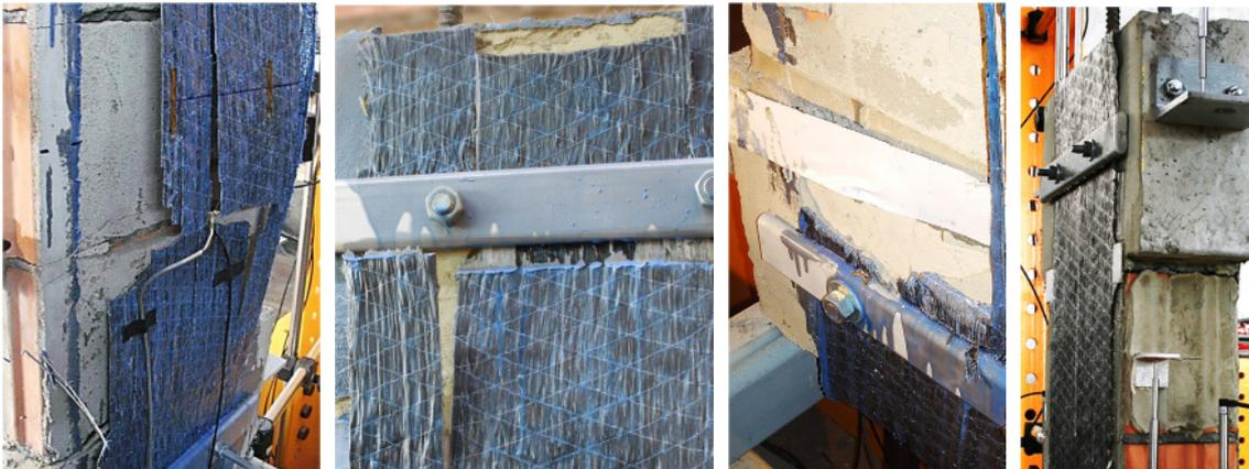
Figures 8a to 8d: Failed specimens F6, F11, and F12 and specimen F9 before failure (from left to right)
