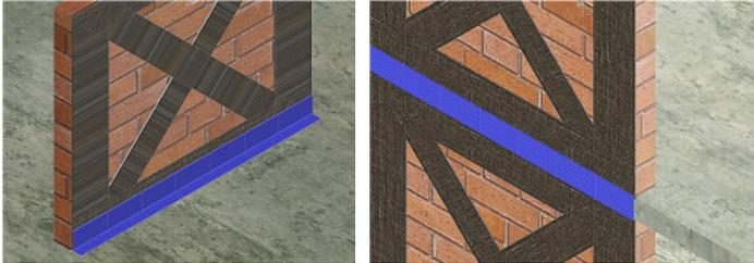
Figures 1a and 1b: Implementation of anchorage for interior walls (left) and for exterior walls (right)
