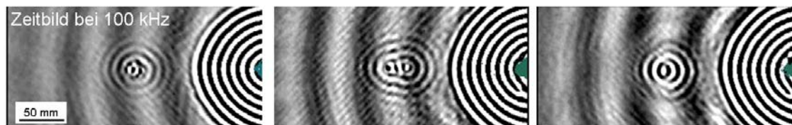
Figure 9: Mode conversion at different types of “damages” (from left: circular and elliptic thickness reductions, circular thickening), see Willberg, Mook et al., 2012.
