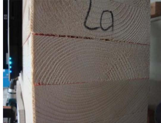
Figure 3. Cross section of missglued middle lamella
