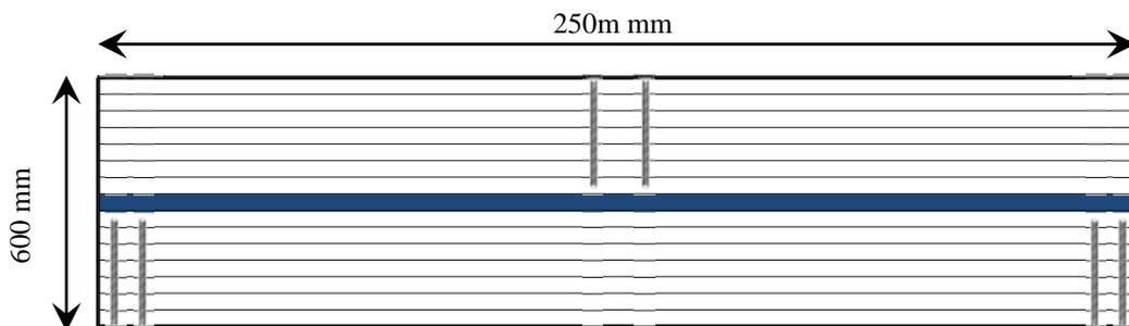
Figure 1. Basic view of the unreinforced specimens. The middle lamella is indicated in dark blue. Both glue-lines of this lamella – the upper and lower one – were missglued over the entire length in such way, that only one third of the glue-line cross-section was available for load transfer. The screws at the supports and the loading point served as reinforcement for the introduction of high loads into the beam.
