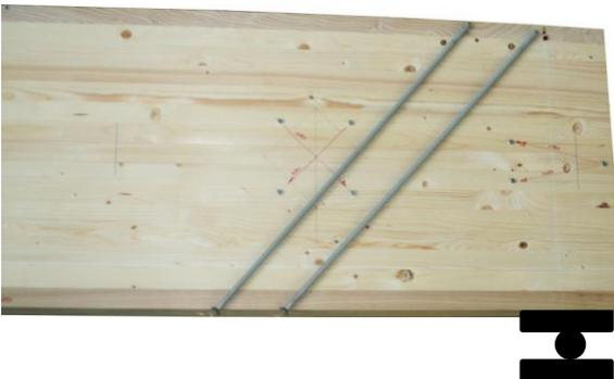
Figure 4. Beam reinforced with screws (demonstration).
