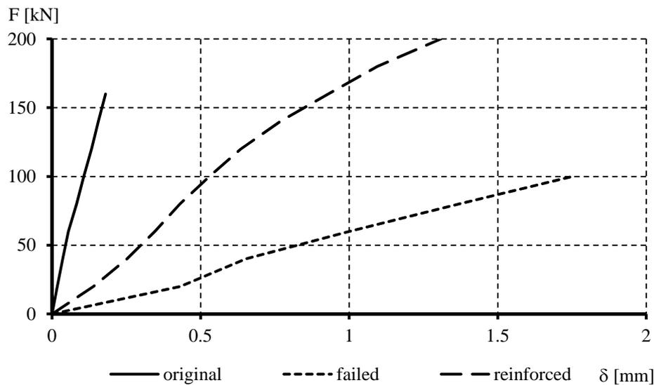
Figure 7. Example for Lamella slip  $\delta$  versus Force  $F$ . The curves show the stiffness obtained for specimen 1b.
