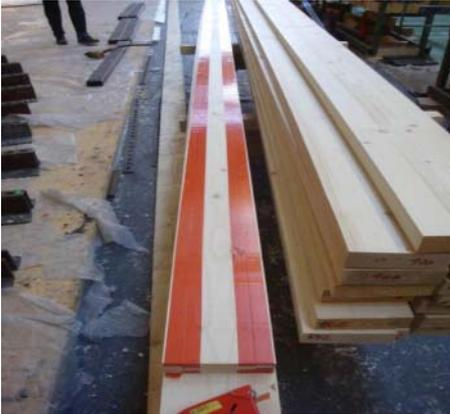
Figure 2. Production of missglued middle lamella at n'H Lungern AG in Switzerland. The surface of the lamella was protected by tape in order to prevent proper wood-wood gluing.
