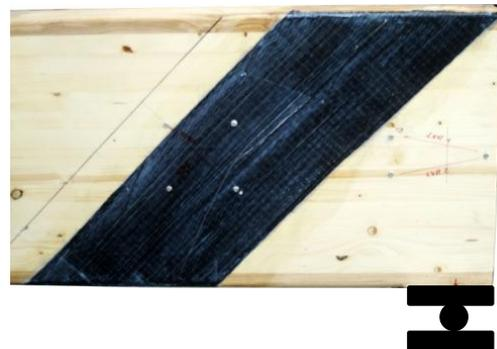
Figure 5. Beam reinforced with unidirectional CFRP sheets
