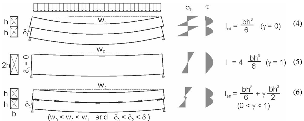
Figure 6. Load bearing behavior of dowelled beams.
