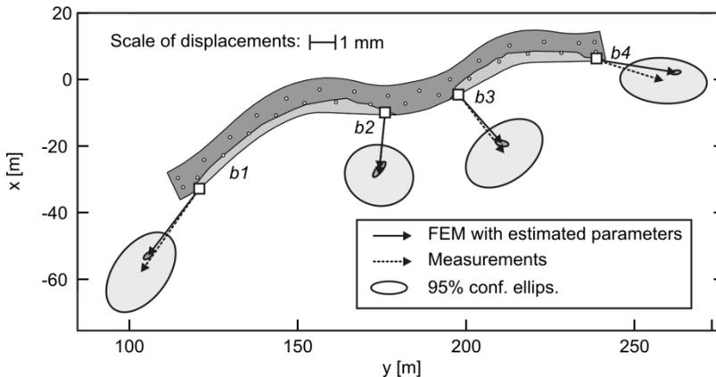
Figure 6. Calculated (calibrated FEM) and measured displacements.
