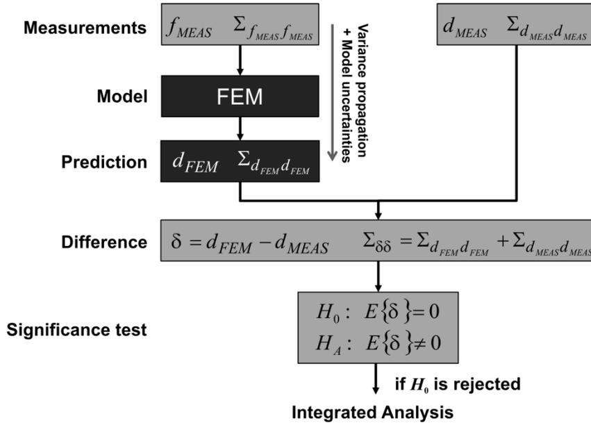
Figure 4. Comparison of calculated and measured deformations.
