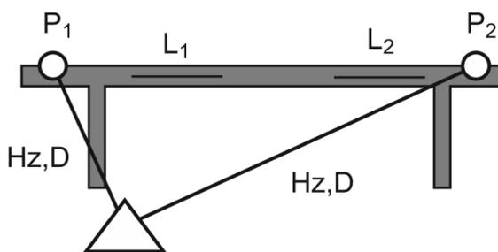
Figure 3. Monitoring example with internal and external measurements.
