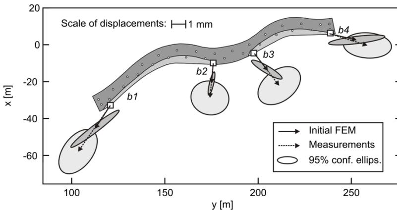
Figure 5. Calculated (initial FEM) and measured displacements.
