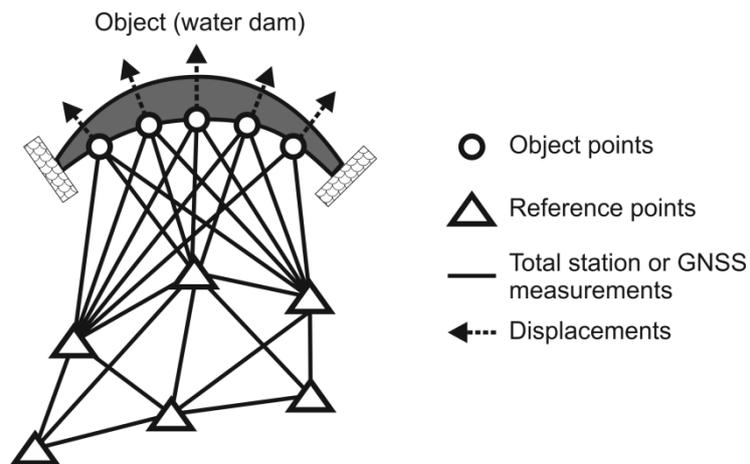
Figure 1. Geodetic monitoring network for a water dam (after Welsch et al., 2000, p. 65).
