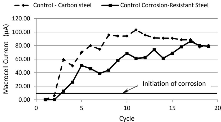
Figure 3: Macrocell current vs. wetting-drying cycle
