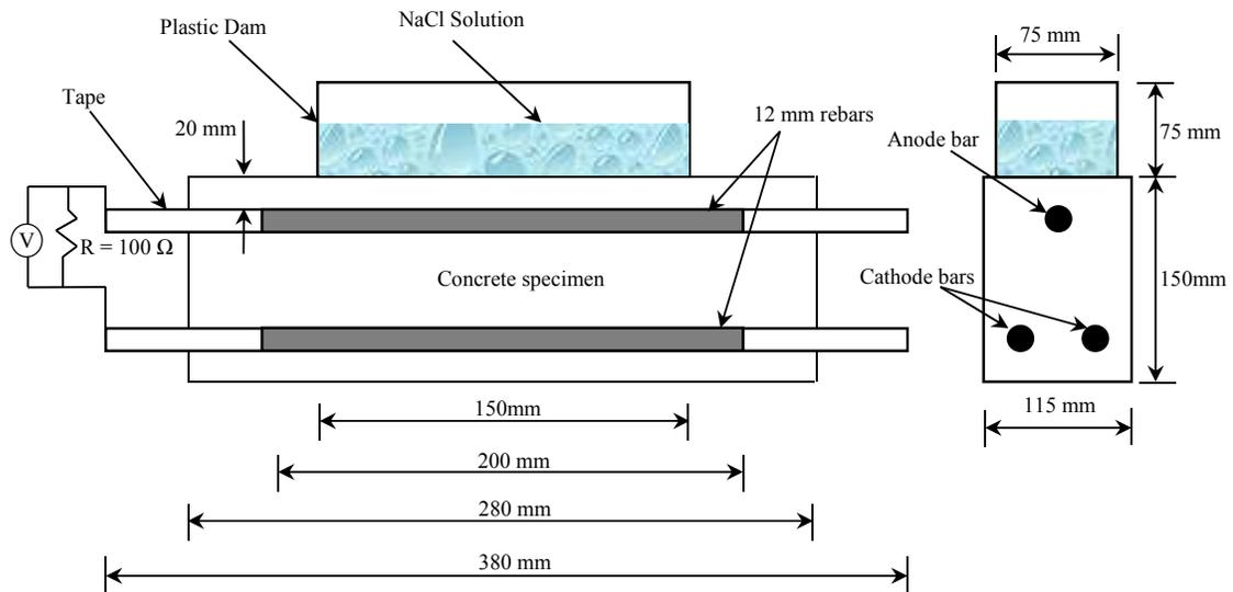
Figure 1: Test setup
