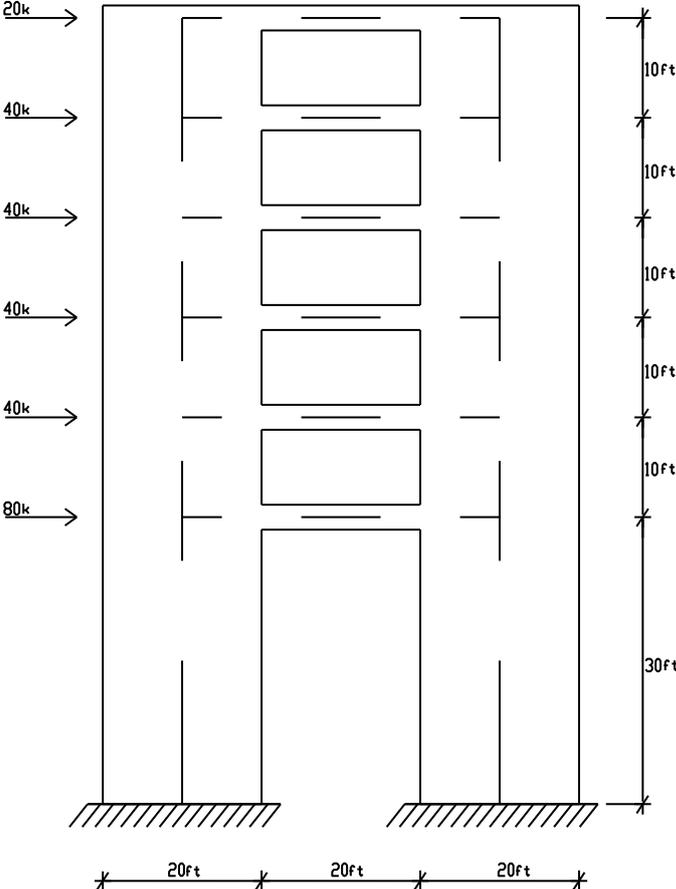
Figure 2(a): Geometry and loading of the example problem.
