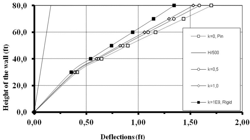
Figure 3: Sway displacements at each floor level in the example problem with varying spring constants  $k$
