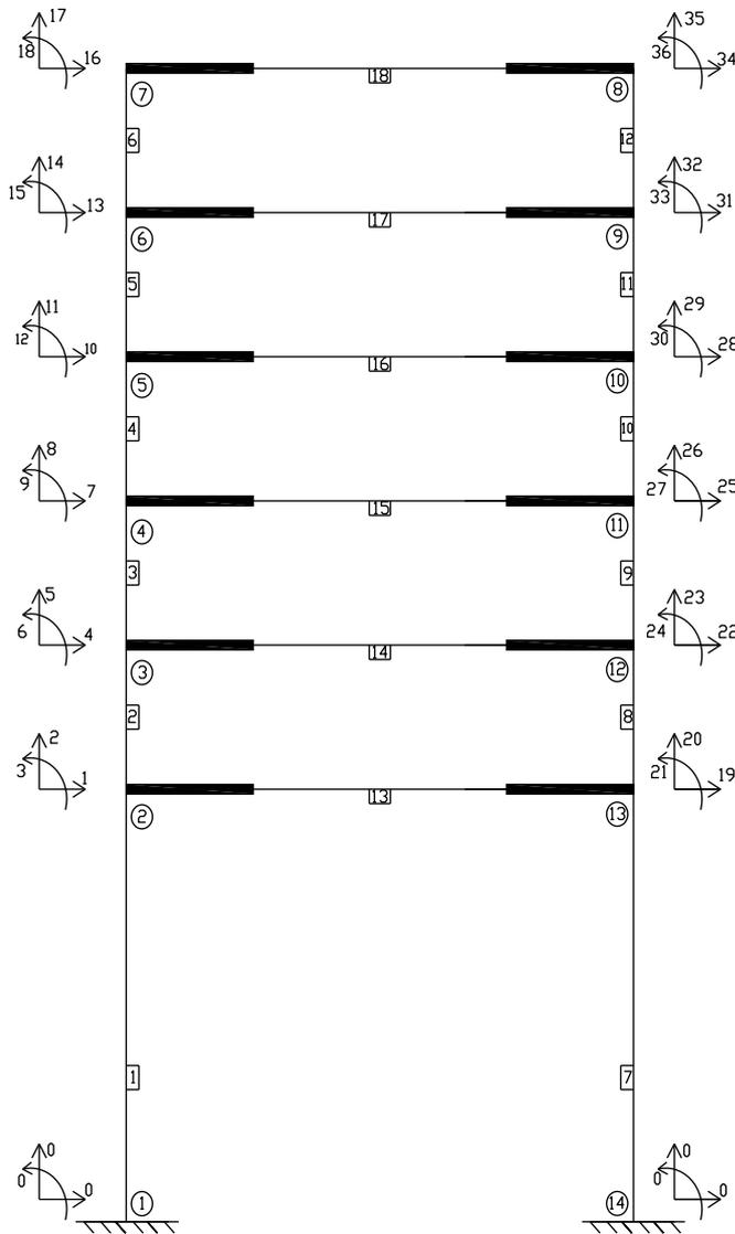
Figure 2(b): Coding and numbering of the example problem.
