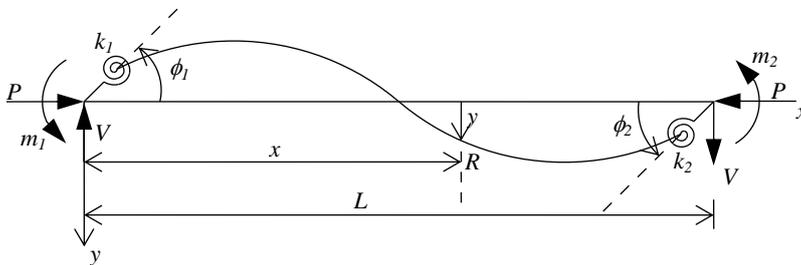
Figure 1: Notation for a member with axial force.
