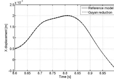
Figure 10b- Zoom on a peak of the transversal displacement response of Pier #1 measured at the cap beam level
