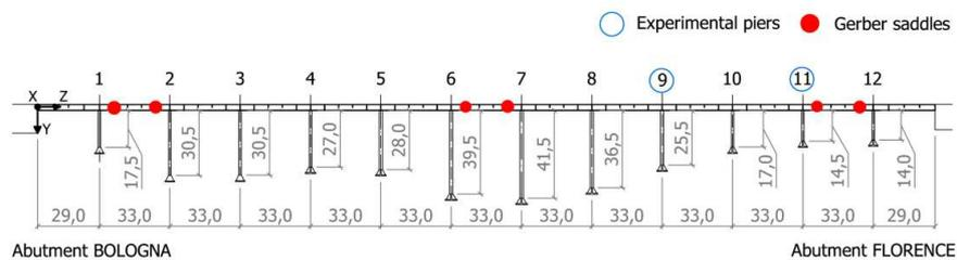
Figure 2. Structural scheme and main dimensions (in m) of the Rio Torto viaduct
