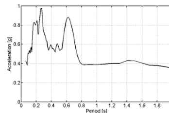
Figure 4b – Acceleration response spectrum of the N-S component of the Emilia earthquake selected for the ULS
