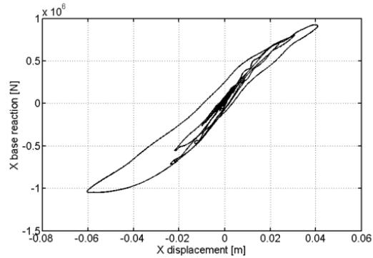
Figure 6b. Transversal base hysteretic loop relevant to Pier #11
