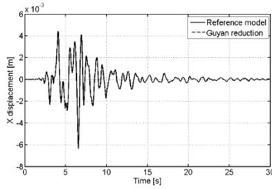
Figure 10a - Transversal displacement response of Pier #1 measured at the cap beam level
