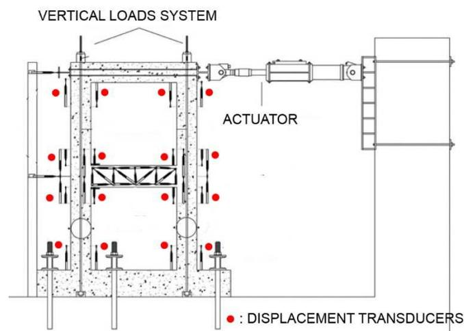
Figure 3. Experimental set-up relevant to Pier #11
