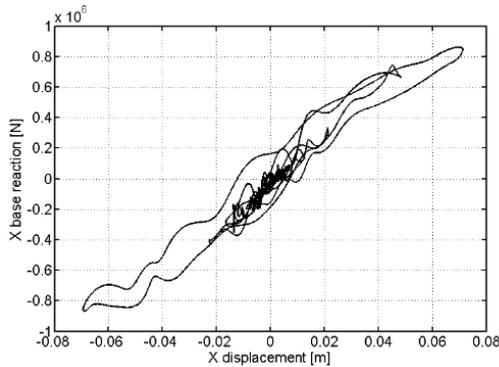
Figure 6a. Transversal base reaction hysteretic loop relevant to Pier #9
