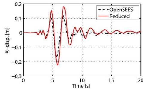
Figure 11b. Transversal displacement response of pier #9 measured at the cap beam level at ULS
