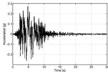
Figure 4a - Accelerogram of the N-S component of the Emilia earthquake selected for the ULS
