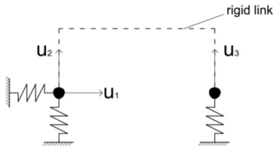
Figure 9 - Pier 3-DoFs superelement geometry
