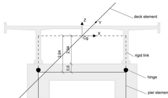
Figure 5. Details of the FE modelling of the pier-deck connection (Dimensions in m)
