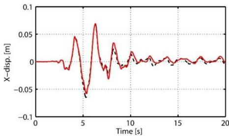
Figure 11a. Transversal displacement response of pier #9 measured at the cap beam level at SLS
