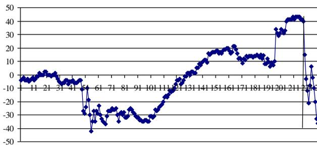
Figure 14. Load history during the hole drilling in terms of strains (vertical axes) vs number of readings
