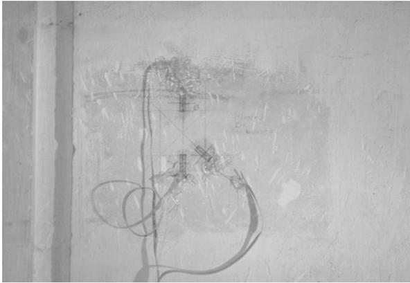
Figure 9. Strain gauges disposition around the point to be investigated
