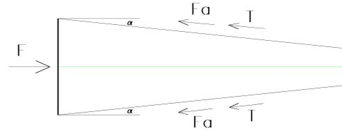
Figure 3. Equilibrium on the central piece of the cylinder
