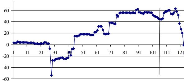
Figure 16. Load history during the hole drilling in terms of strains (vertical axes) vs. no. of readings
