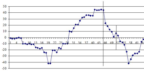
Figure 12. Load history during the hole drilling in terms of strains (vertical axes) vs number of readings
