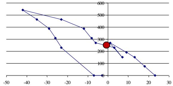
Figure 13. Load [kN] strains [µm/m] curve for SG1 in D1 pillar
