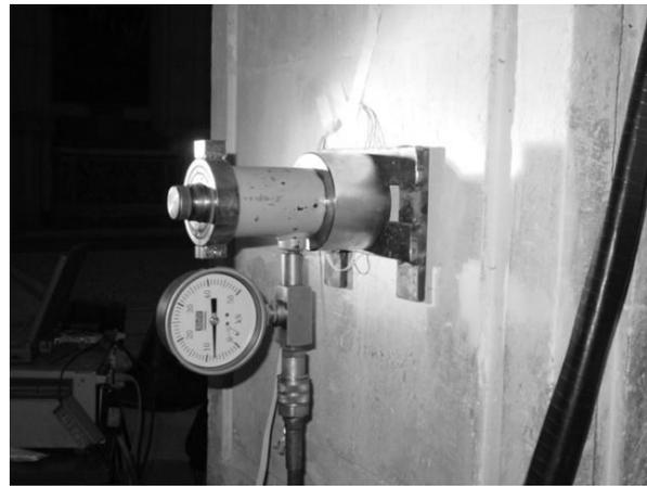
Figure 11. Instrument disposition in the hole and test equipment for the load measurement
