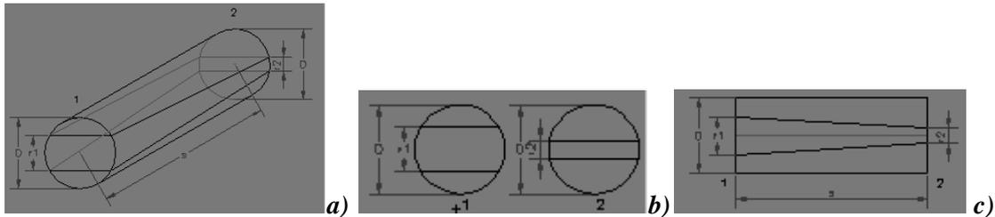
Figure 1. Shape of the proposed dilatometer a) axonometric; b) frontal section; c)lateral section.
