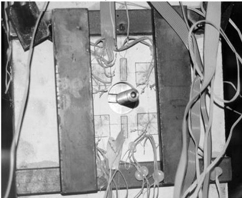
Figure 4. Dilatometer view inside the brick hole
