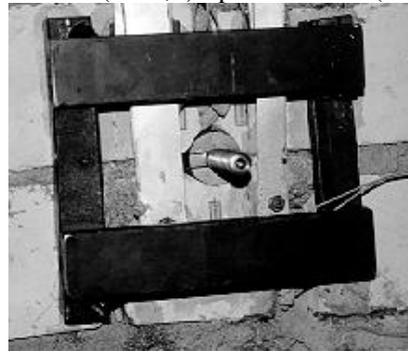
Figure 7. Dilatometer test on the masonry
