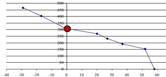
Figure 17. Load [kN] vs. strains [µm/m] curve for SG2 in D3 pillar
