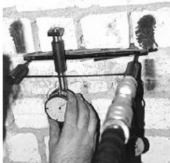
Figure 6. Flat jack test on the masonry
