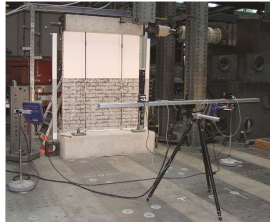
Figure 3. 3D image correlation system installation of Wall 4.
