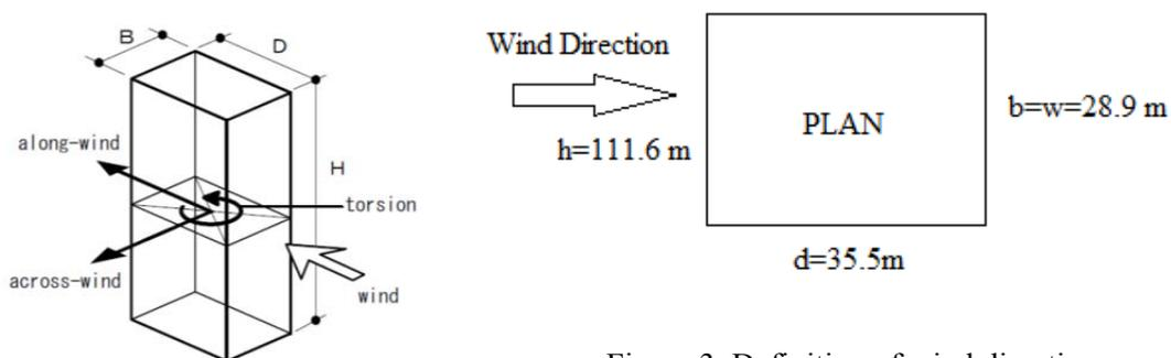
Figure 3. Definition of wind direction
