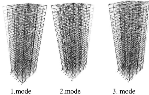
Figure 2. The first three mode shapes of building
