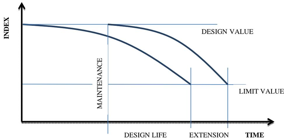
Figure 1. Typical lifetime function and the effect of maintenance.
