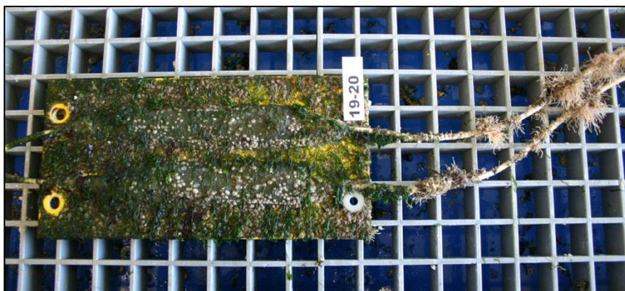
Figure 6. Detailed view of one of the exposed sensor-equipped plates. Clearly can be seen the marine biology vegetation (algae, barnacles and polyps at the leading cable).
