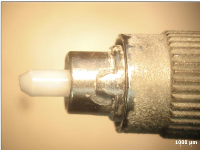
Figure 4. Connector corroded by salt-water influence during salt-water attack test.
