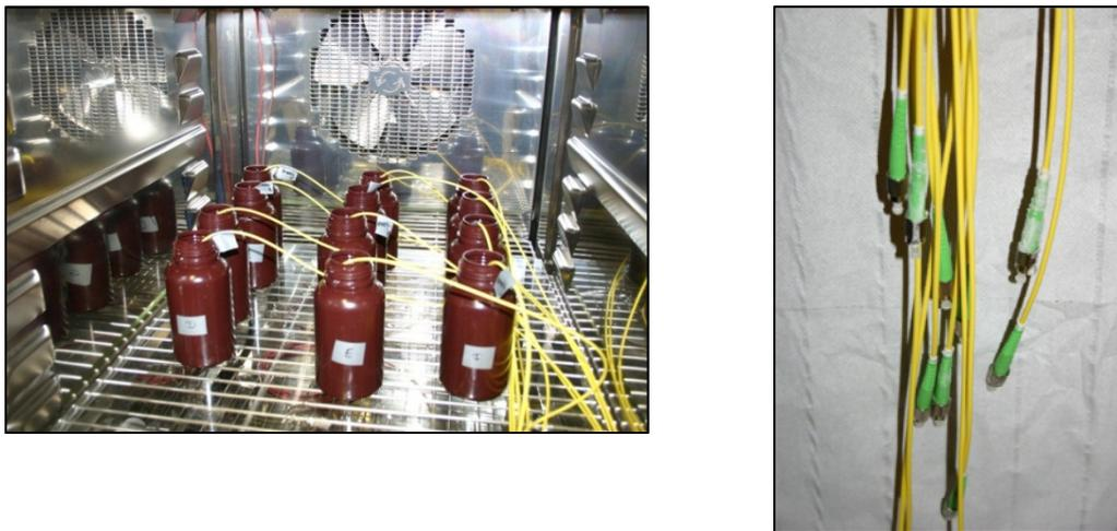
Figure 1. Climate chamber to test optical cables under salt-water influence. The picture right shows the connectorized cable ends.
