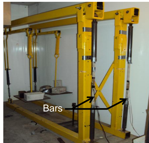
Figure 10. Conditioned tensile test setup of GFRP bars.
