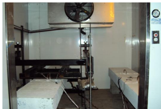
Figure 2. The environmental room including the four point flexural setup, slabs SA and SB.
