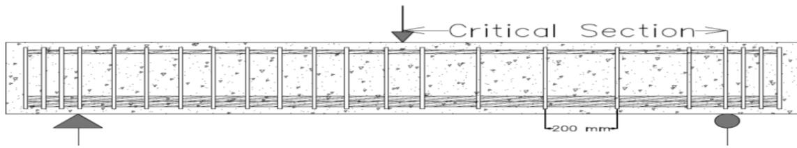
b) Reinforcement layout along the span
