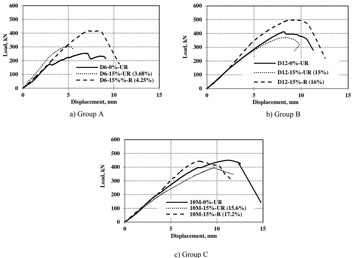
Figure 6 Load-displacement responses of beams in group A, B, C
