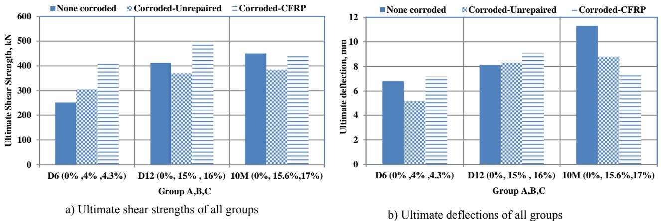
Figure 7 Effect of CFRP repair on shear strength and deflection
