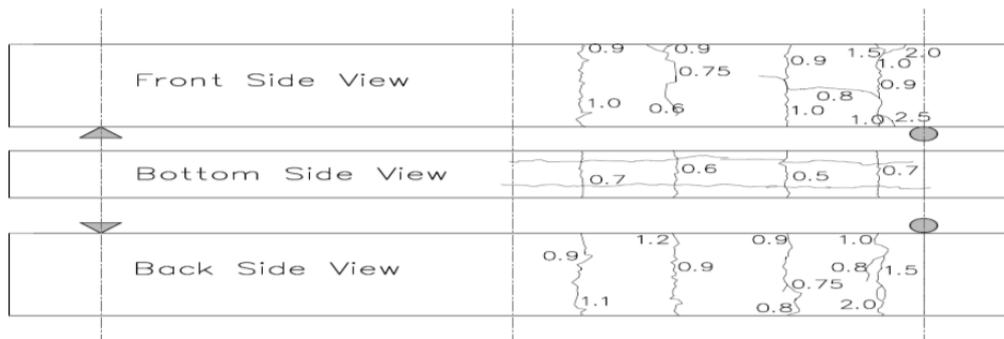
Figure 4 Typical patterns of corrosion cracking (crack width in mm)
