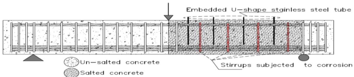
Figure 2 Corroded beam geometry and reinforcement details
