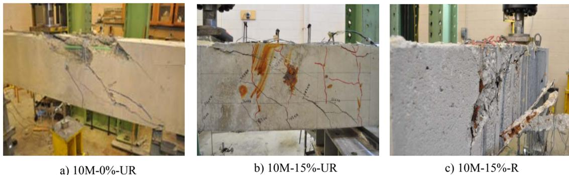
Figure 5 Failure modes of beams in group C
