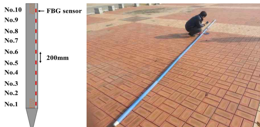
Figure 4. The manufactured instrument for installing in the river and the position of FBG sensors
