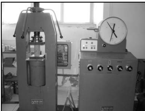
Figure 3. Compressive testing machine.
