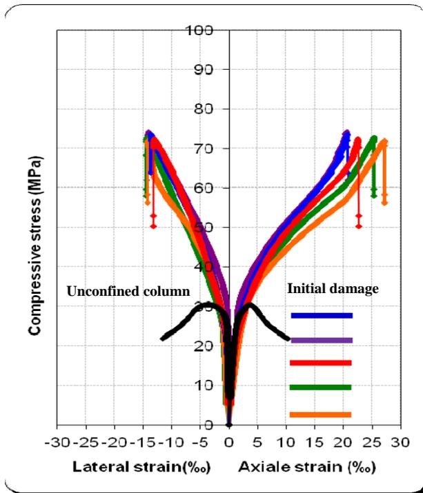
Figure 4: Stress strain curves for repaired specimens
