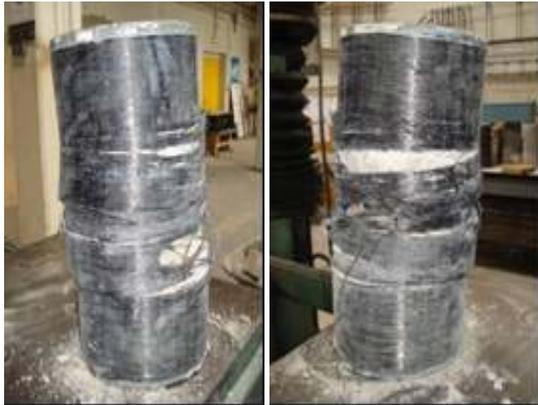
Figure 2. Failure of CFRP confined specimens
