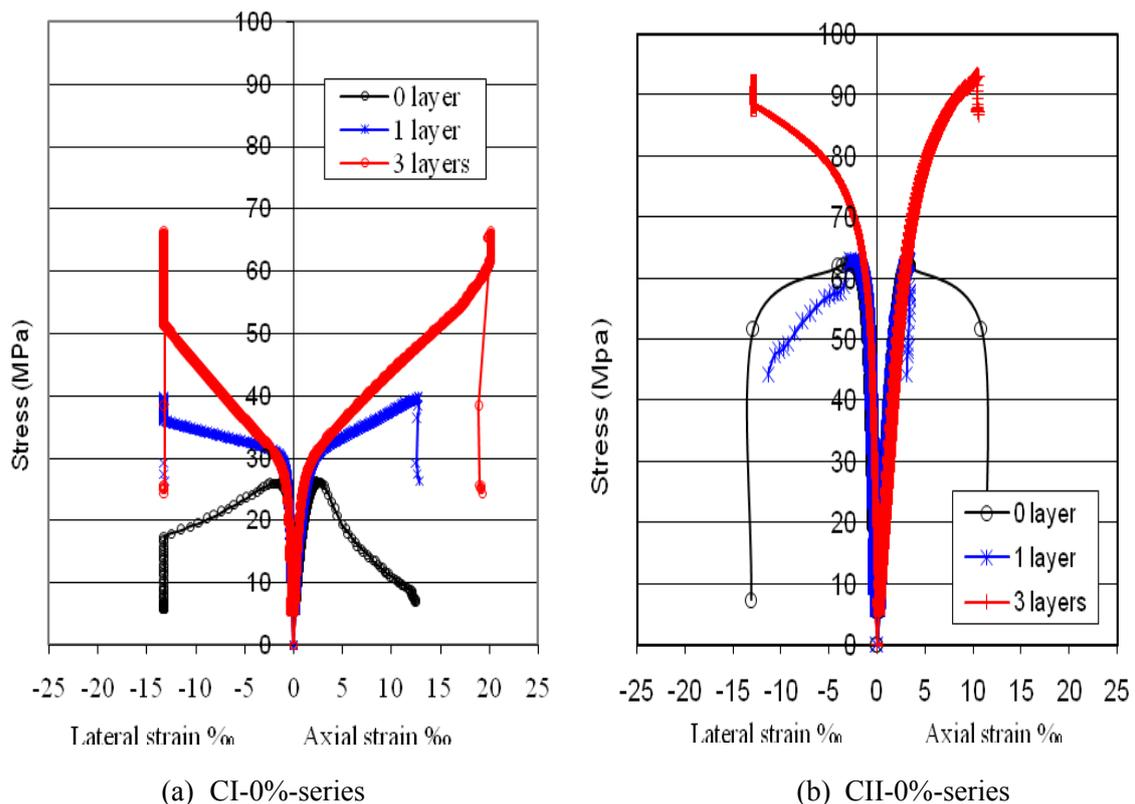
Figure 3: Stress strain curves for strengthened specimens
