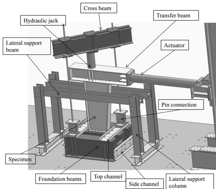
Figure 2. Test setup.
