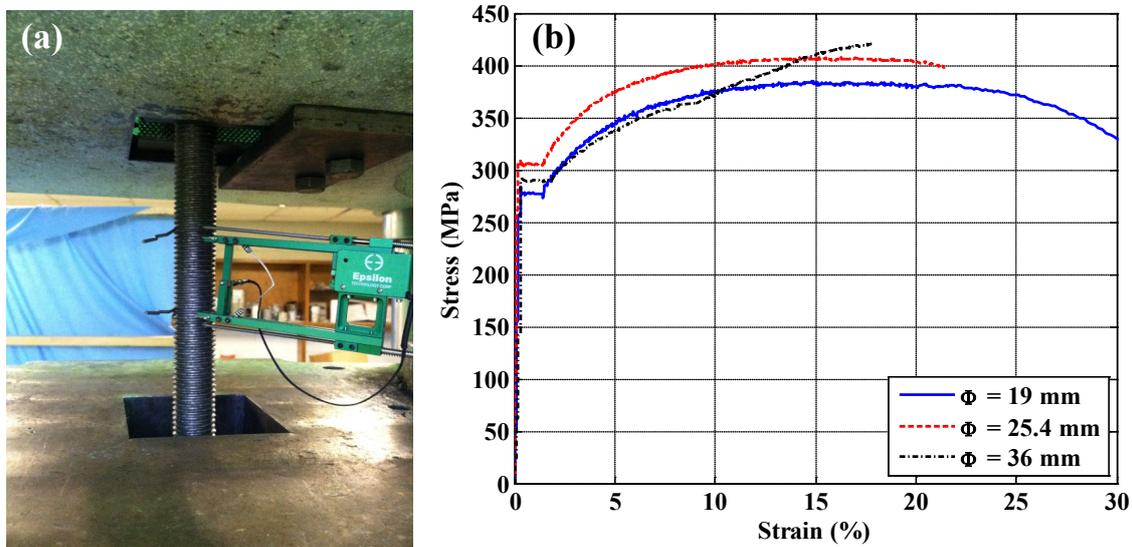
Figure 4. (a) Tensile testing of anchor rods, (b) stress-strain curves for different diameter anchor rods
