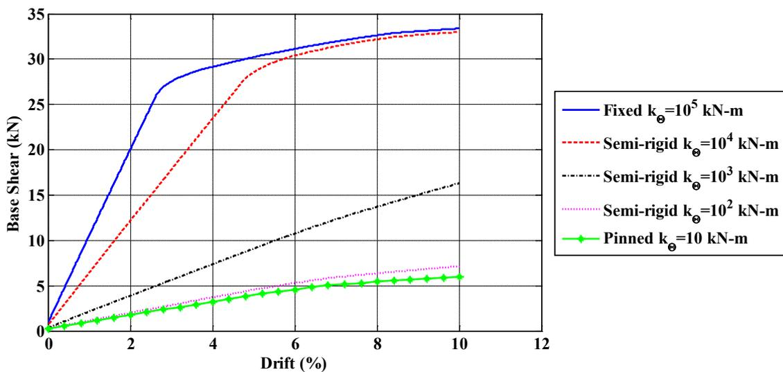
Figure 6. Base shear vs. interstory drift curves for rigid, semi-rigid and pinned base connections.
