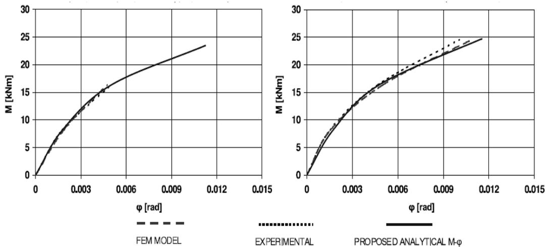
Figure 8. A comparison of moment-rotation curves of two specimens based on analytical formulas given in Eqn (1), FEM models and experiments (Stamatopoulos, 2011)
