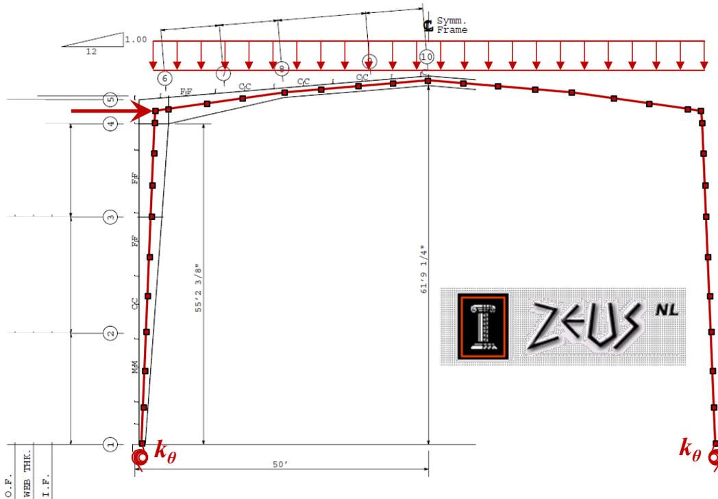
Figure 5. Long span steel tapered section frame models for finite element analysis using ZEUS NL (Elnashai et al., 2010).
