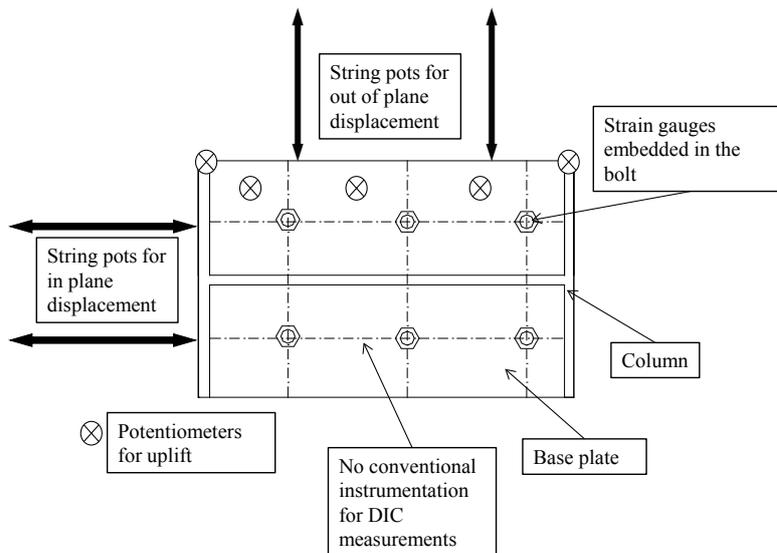
Figure 3. In plane and out of plane measurements
