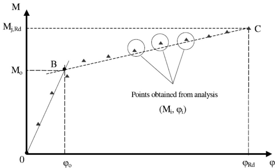
Figure 7. Moment-rotation curve obtained using Eqn. (1) [Ermopoulos, 1996]
