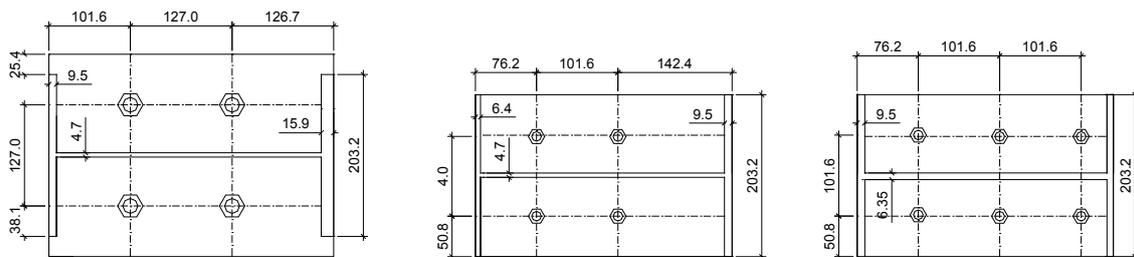
Figure 1. Typical configuration of base plates (all dimensions are in mm)
