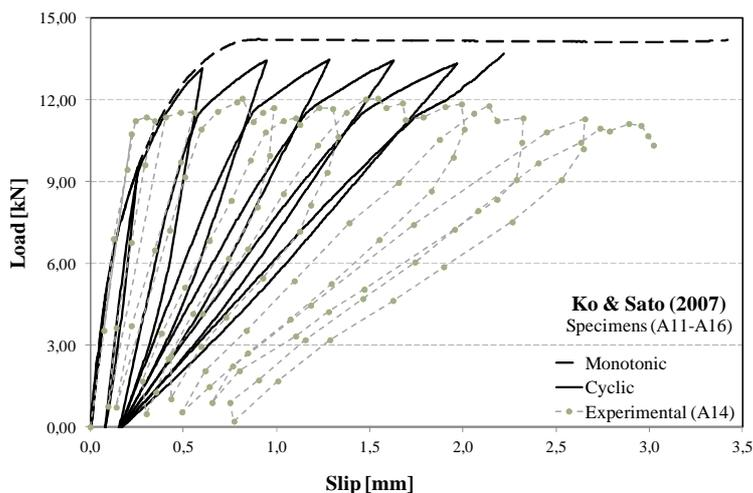
Figure 5. Load-slip response under monotonic and cyclic actions of FRP strips glued on concrete (Ko & Sato, 2007) – Linear softening.
