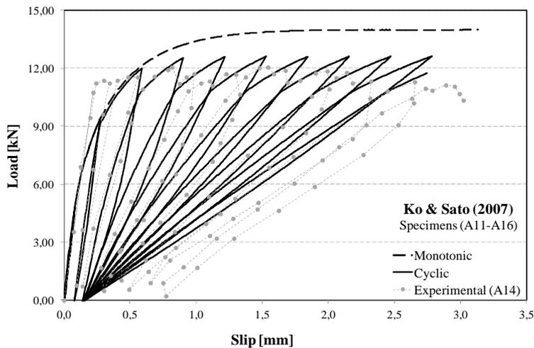
Figure 4. Load-slip response under monotonic and cyclic actions of FRP strips glued on concrete (Ko & Sato, 2007) – Exponential softening.
