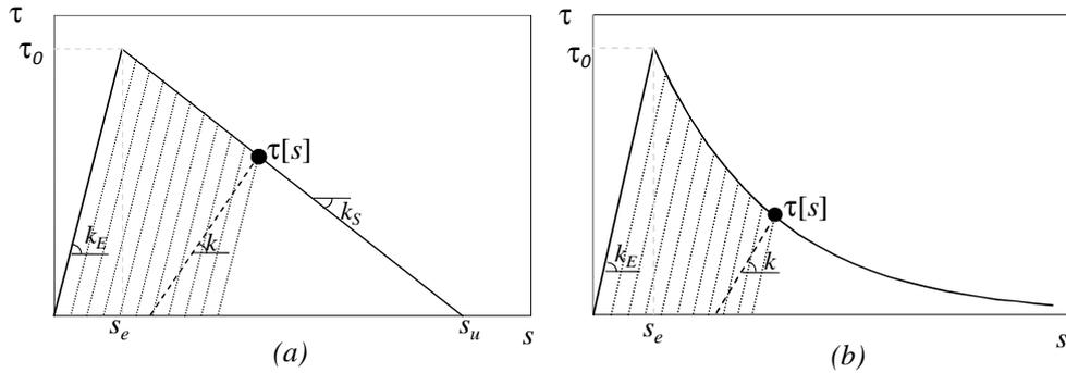
Figure 2. Fracture work spent as defined in eq. (6): (a) linear and (b) exponential softening branches.
