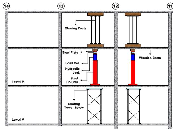
**Figure 3. Test Setup**
