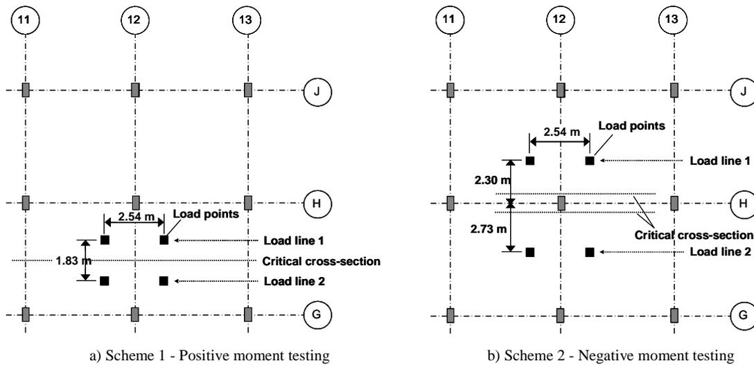
**Figure 2. Load Test Schemes and Point Loads Layout**
