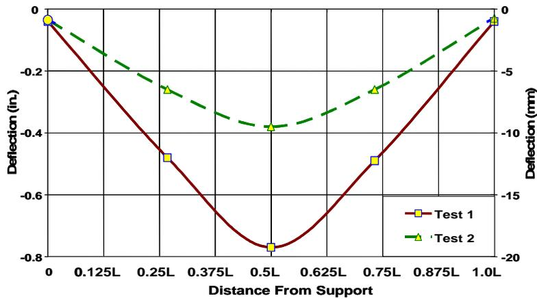
**Figure 6. Comparison of Measured Deflections at P = 64.5 kN**
