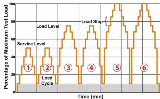
**Figure 1. Typical Load Cycles**
