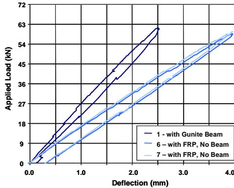
Figure 10. Load deflection for Tests 1, 6 & 7.
