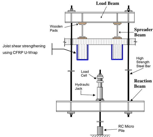
**Figure 5. Cyclic Load Test Setup for Test 1 and Test 2**
