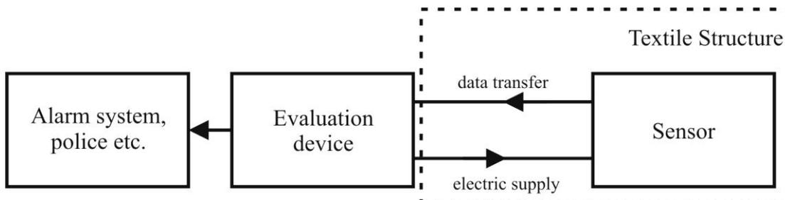
Figure 3: Principle operation of monitoring systems
