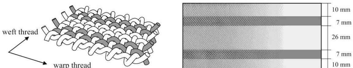
Figure 4: Example of produced conductive narrow fabric (NF 3)
