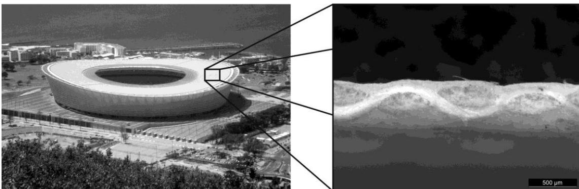
Figure 1: World Cup soccer stadium in Cape Town, SA (left) and microscopic cross section of used PTFE-coated glass fabric (right)
