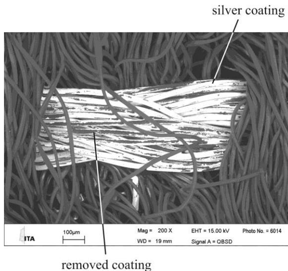
Figure 8: SEM picture of silver coated Polyamide 66 filaments of narrow fabric 3 after 20 washes
