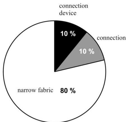
Figure 6: Percentage of connection parts of the overall electrical resistance
