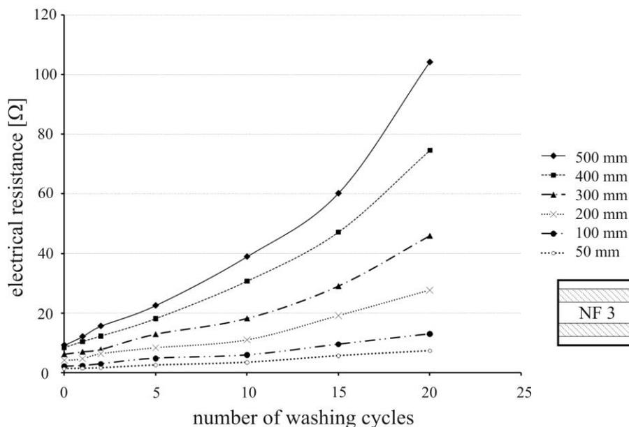
Figure 7: Effect of washing on electrical resistance of narrow fabric 3 at different distances
