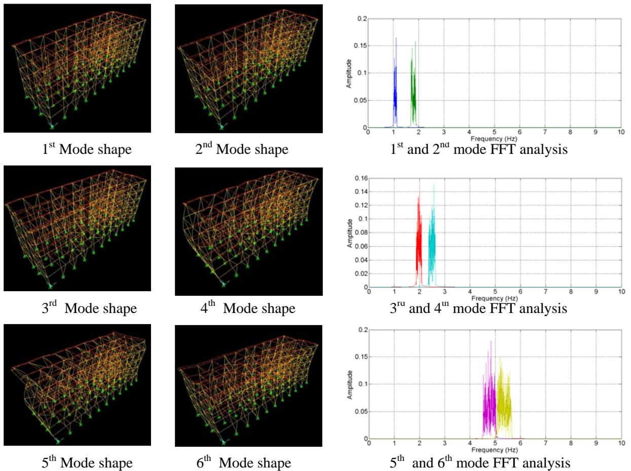
Figure 4. First six structural mode shapes and FFT analysis results
