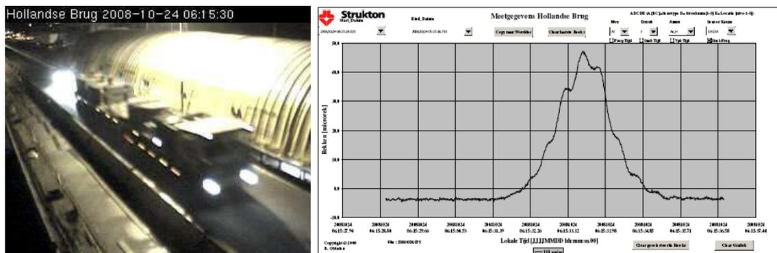
Figure 6. Left: Image of ballast truck 100 mT; Right: Strain registration of main girder during passing.
