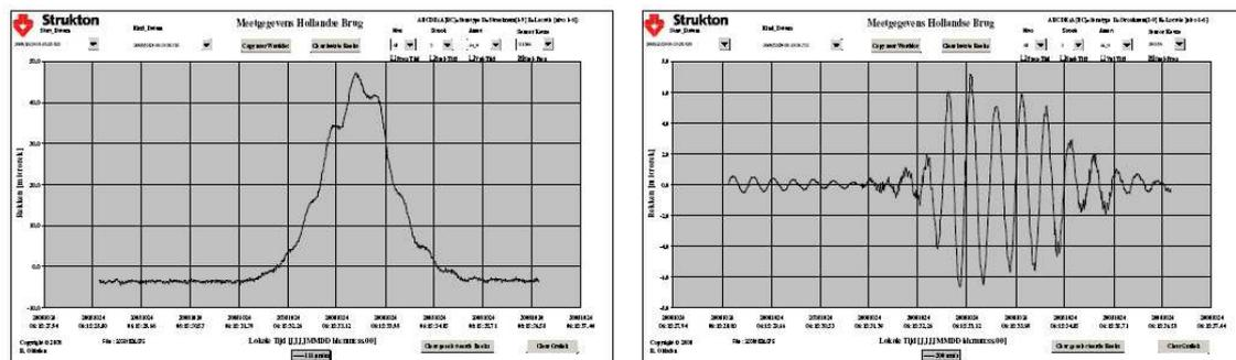
Figure 5. Data capture of strain (Left) and particle velocity (Right) of a large truck crossing the bridge.
