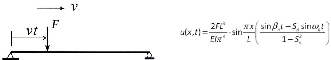
Figure 2. Left: mathematical scheme of the dynamic model; Right: formula describing the response of an elastic beam under a moving load.
