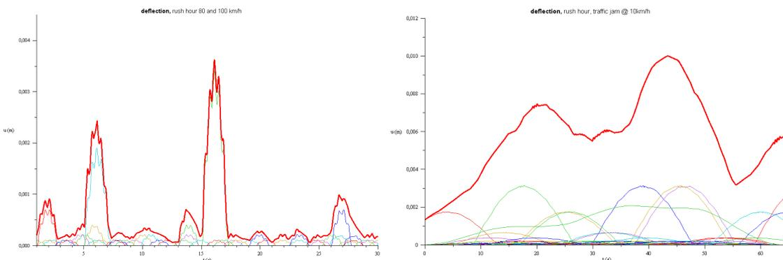
Figure 3. Left: Case 1) Typical deflection during intensive traffic including heavy cargo vehicles; Right: Case 2) Typical deflection during congestion.
