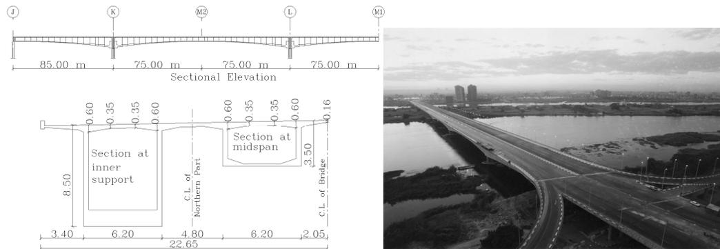
Figure 1. Sectional elevation, cross section, and a photo-El Moneeb Bridge
