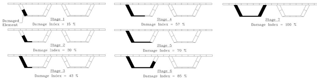
Figure 8. Crack progress in the box section bridge
