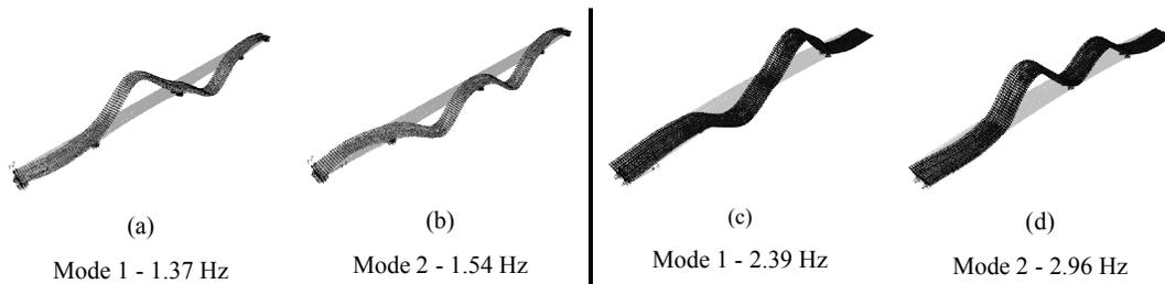
Figure 4. (a) & (b) are El Moneeb Bridge's first and second bending modes; (c) & (d) are Thuwal Interchange Bridge's first and second bending modes
