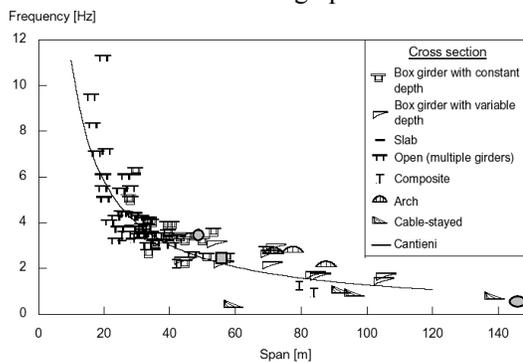
Figure 6. Fundamental frequency as a function in span length
