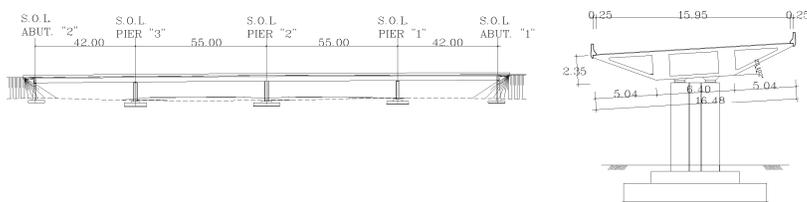
Figure 2. Sectional elevation and cross section-Thuwal Interchange Bridge
