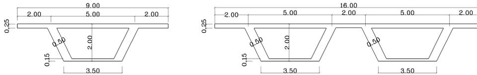
Figure 7. Cross sections of the bridge models
