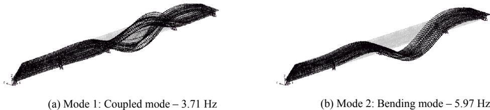
Figure 5. El Matar Bridge's first mode and second mode
