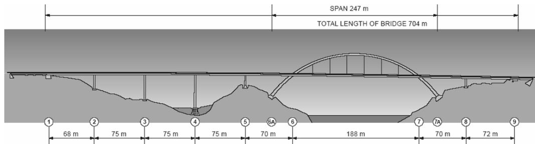
Figure 1. Sketch of the New Svinesund Bridge in its entirety, showing gridline numbering and dimensions.
