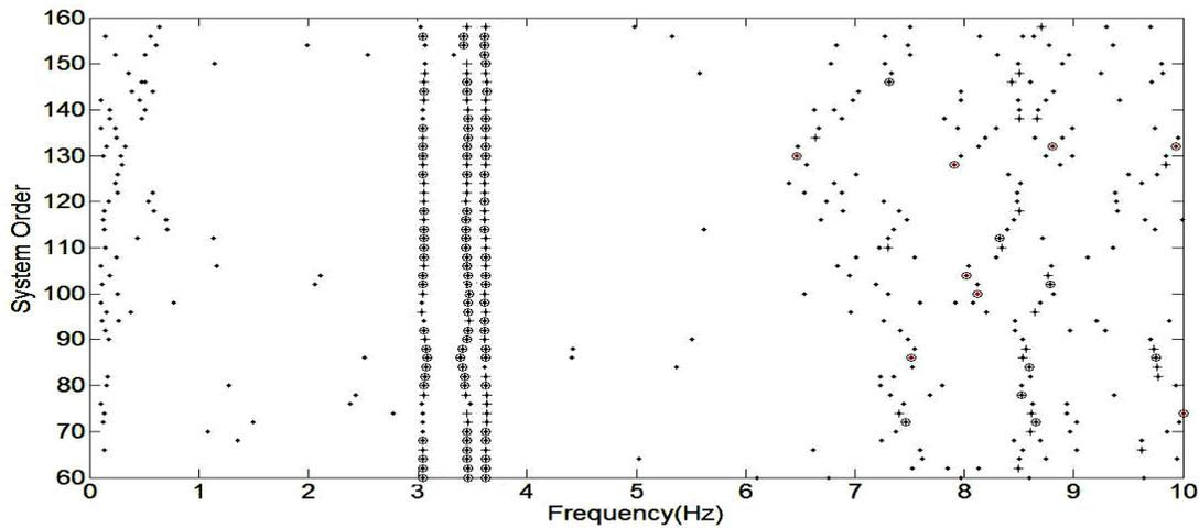
Figure 4. Stabilization diagram showing the trends of frequencies. Marker sign “dot” shows all the identified frequencies, “plus” sign the stable frequency and damping ratio, while “plus with circle” sign the stable frequency with damping ratio and mode shapes.
