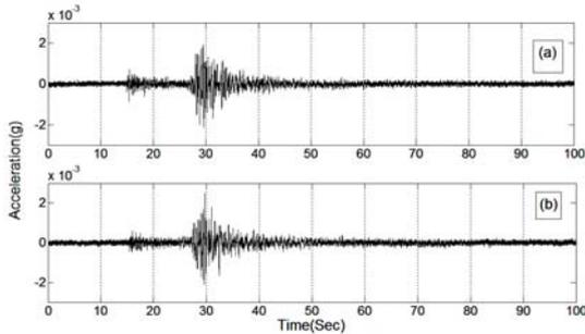
Figure 2. Building base seismic acceleration time histories from sensor 6: (a) EW-component (b) NS-component (PGA).
