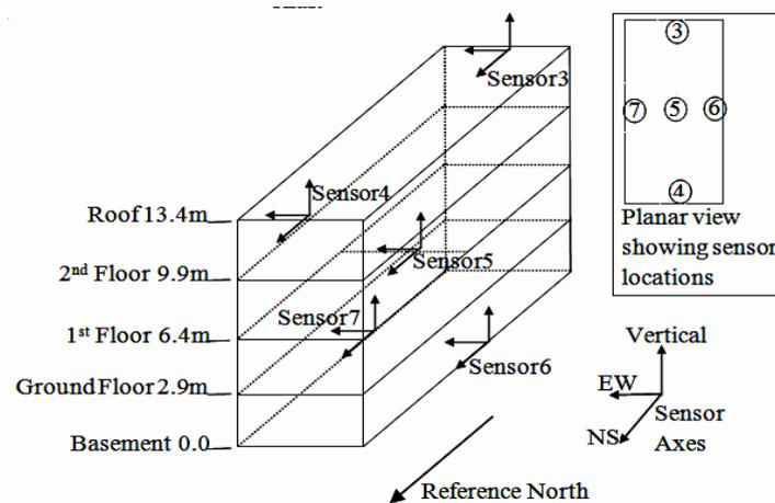
Figure 1. Three dimensional sketch of the building showing sensor array marked with sensor numbers and their sensitive axes. Inset shows a planar view marked with sensor locations.
