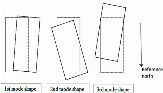
Figure 5. Planar views of the first three mode shapes identified using subspace state-space identification method.
