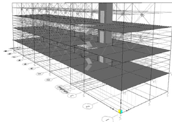
Figure 6. Three dimensional FEM showing shear core, soil springs, partition walls and stairs. Cladding has been removed from the view to show the inner details.
