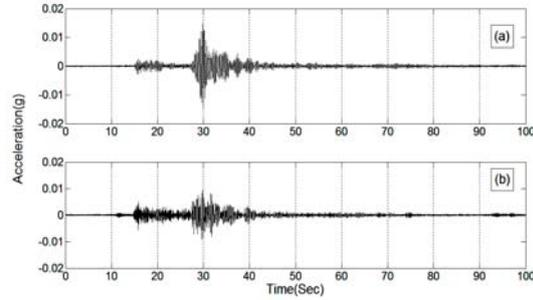
Figure 3. Building roof seismic acceleration time histories from sensor 4: (a) EW-component (PRA) (b) NS-component.
