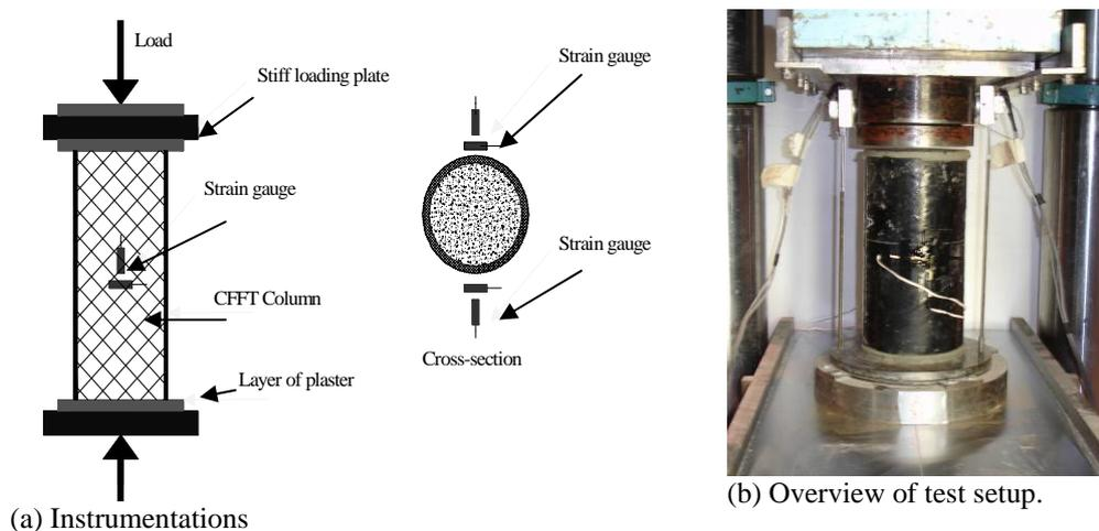
Figure 4. The instrumentations and test setup.
