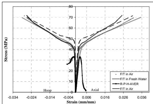
Figure 7. Stress strain curves of conditioned and unconditioned CFFT specimens. Each of the curves presents the average of three tested specimens.
