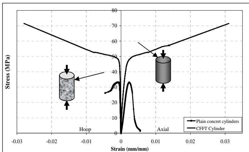
Figure. 5 Typical stress strain curve of unconfined and confined specimens.
