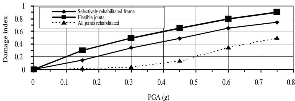
Figure 7. Damage relationship for the 3-story frames due to the El Centro earthquake scaled to different PGA.
