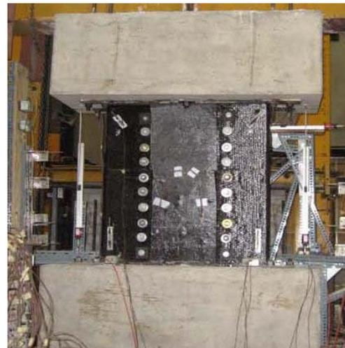
Figure 4. Front view of the rehabilitated wall
