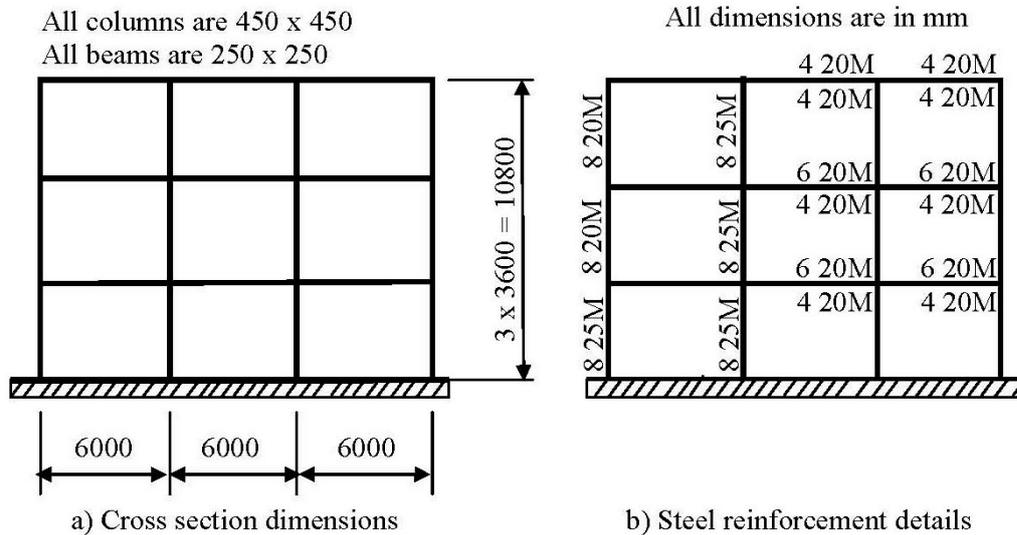
Figure 5. Dimensions and reinforcement of the three-story frame.
