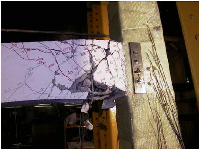
Figure 3. Beam hinging in a rehabilitated joint.
