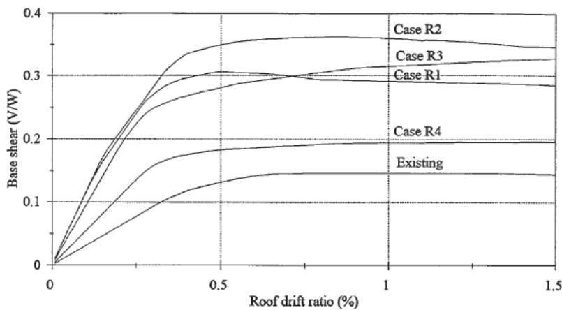
Figure 10. Performance curves of the various rehabilitation cases from the pushover analysis.
