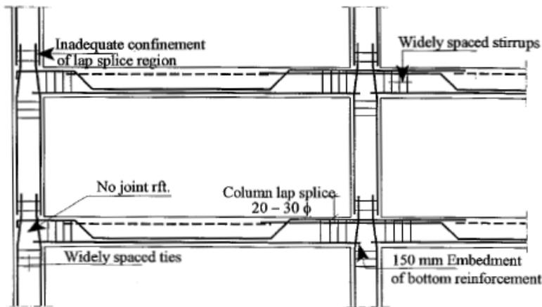
Figure 1. Typical deficiency in existing moment resisting frames.
