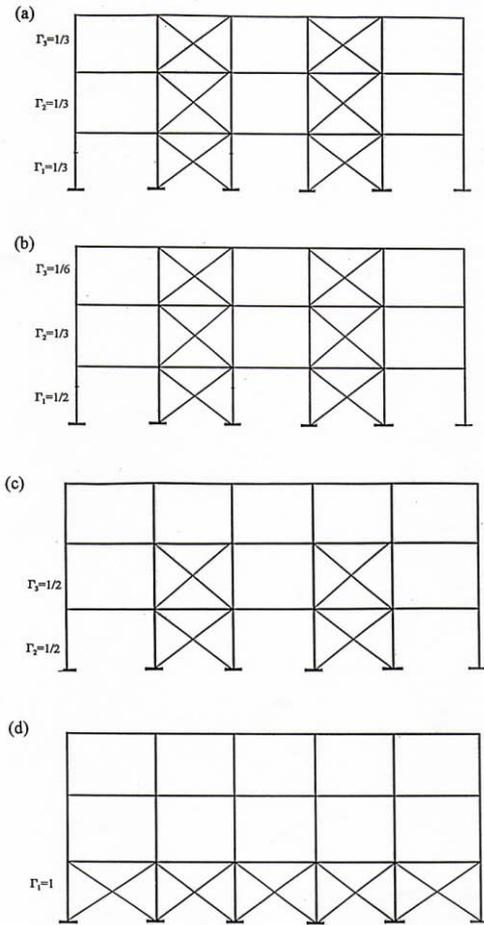
Figure 9. Rehabilitation cases for nonductile 3-story building: (a) case R1; (b) case R2; (c) case R3; (d) case R4.
