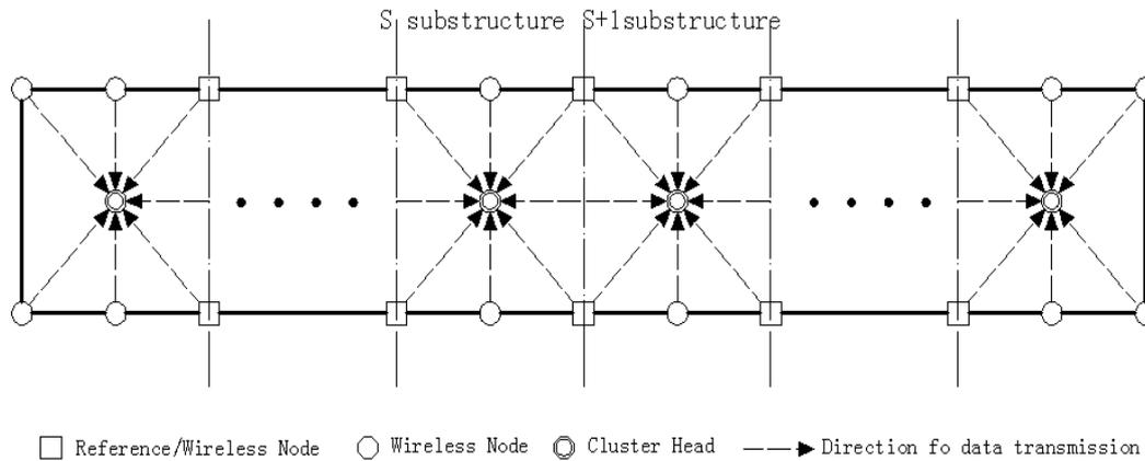
Fig. 5: Distributed computing strategy of modal identification with wireless sensing network
