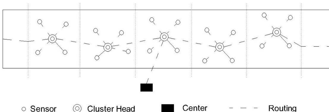
Fig.1: A cluster-tree wireless network topology of the new wireless sensor network
