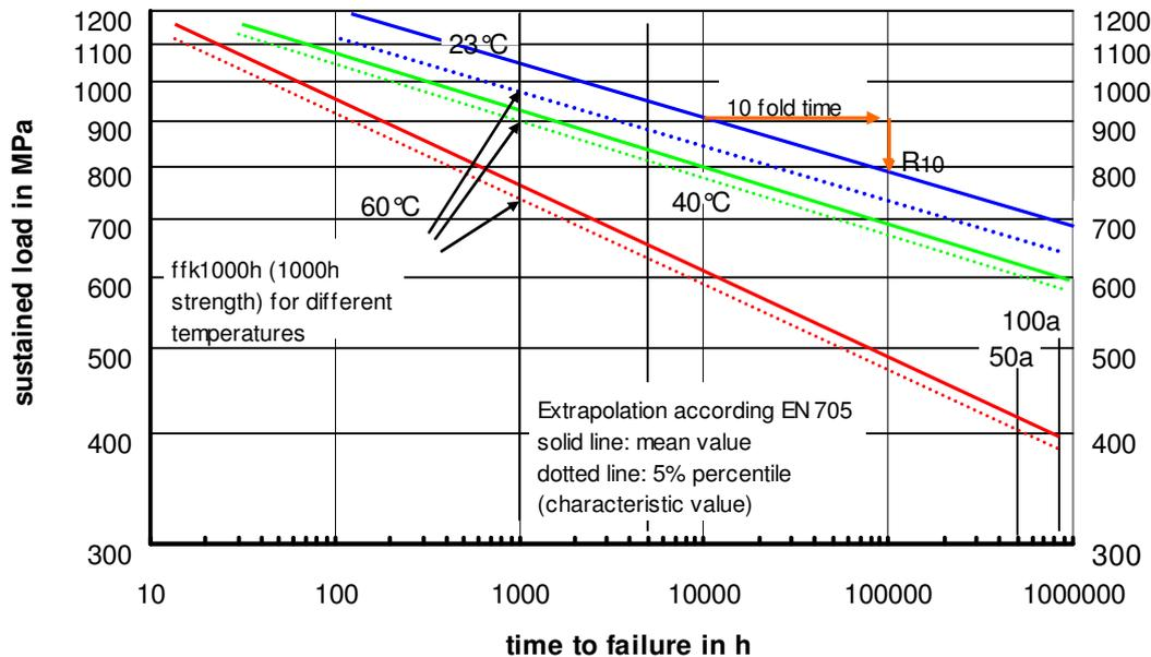
Figure 4. Time to Failure Lines for ComBAR Bars at various Temperature Levels
