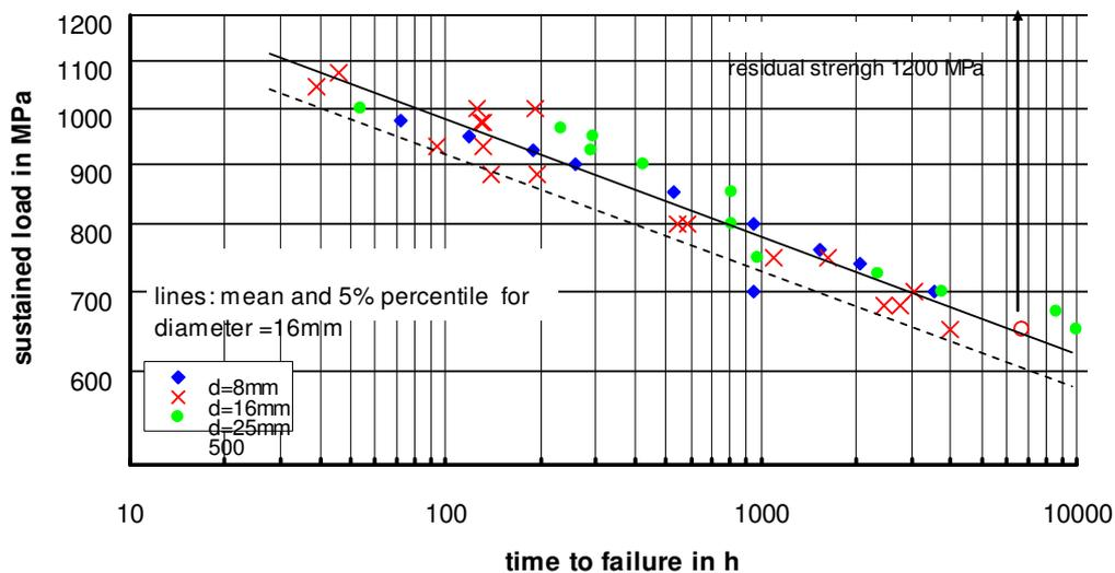
Figure 3. Long-term Tensile Tests under Load: Time to Failure Line (60°C, wet concrete )
