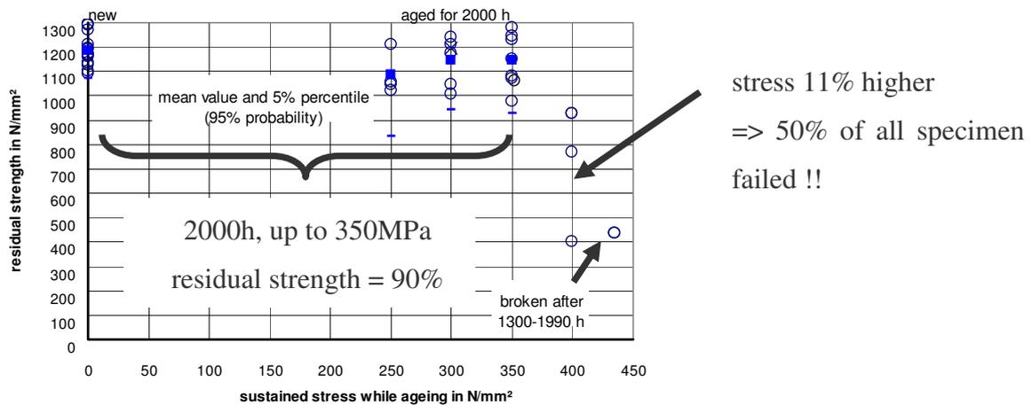
Figure 1. Stress Threshold in Residual Testing
