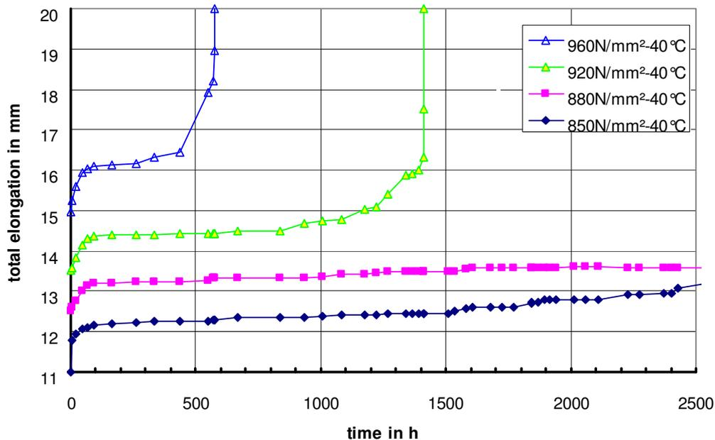
Figure 2: Creep rupture curves for constant Load until Rupture (Ø 16mm bar, wet concrete, 40°C)
