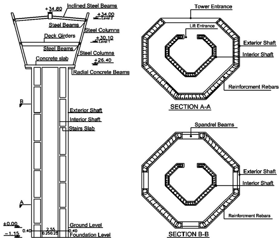
Figure 2. Longitudinal and cross-sections of Kerman ATC tower.
