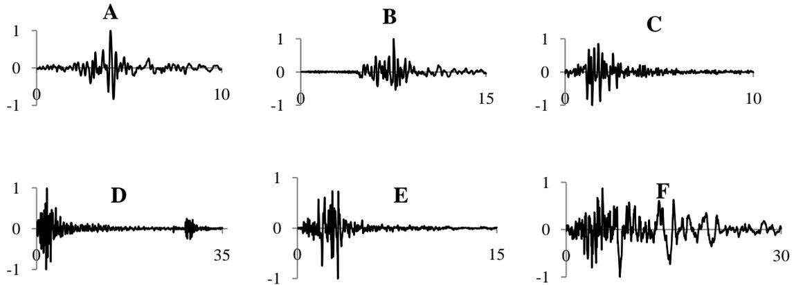
Figure 3. Applied earthquake records for nonlinear time history analysis.
