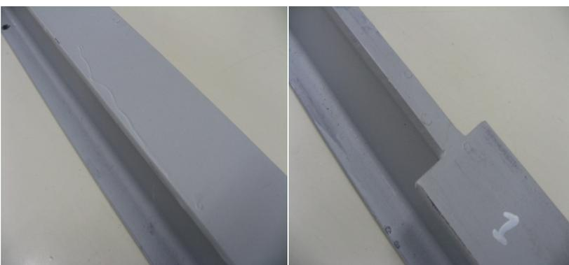
(b) Main girder without damage (c) Main girder with damage in lower flange
