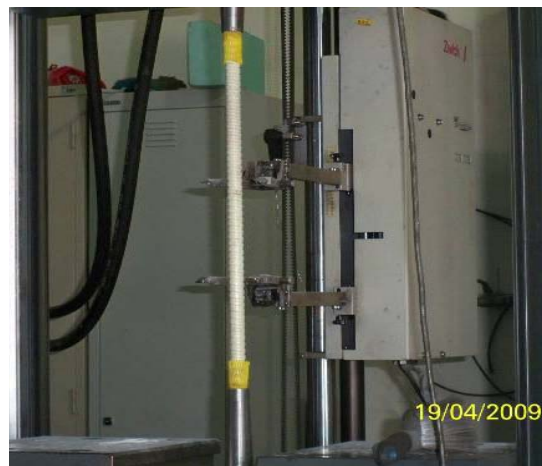
(b) 16 mm diameter specimen loaded in the machine
