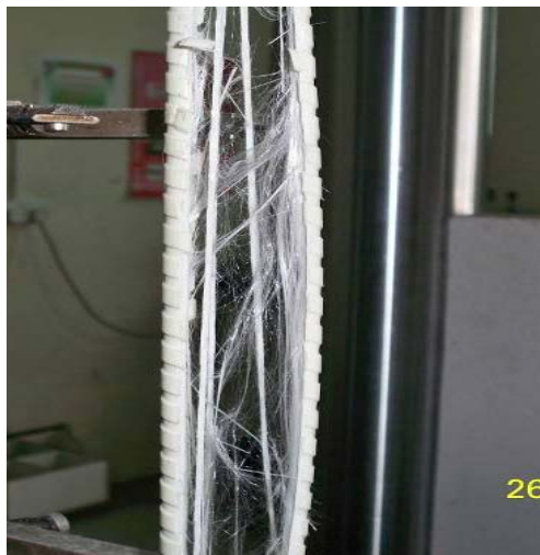
(c) initial split of the specimen
