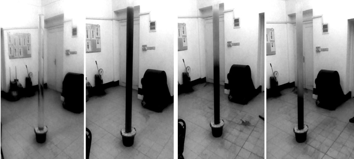
Fig 1 Test Setup showing test tube filled with water and sedimentation process of cement paste (Phase I)
