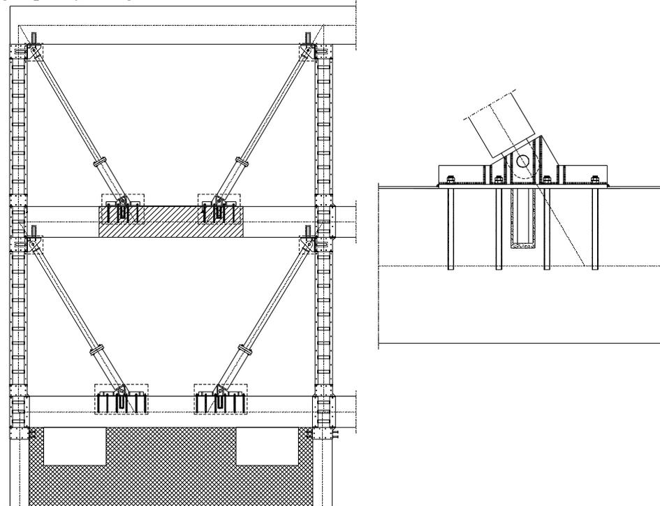
Figure 4. Seismic details for the bays of the frame incorporating unbonded braces.
