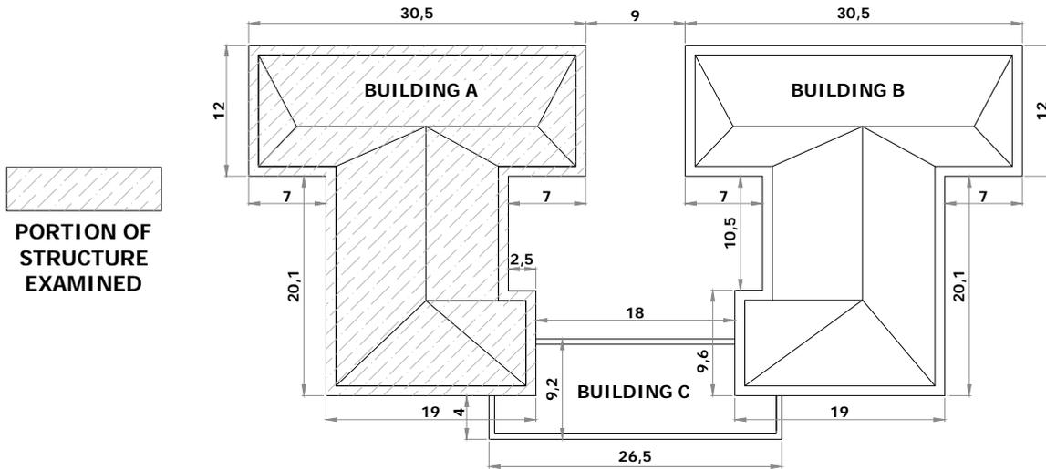
Figure 1. Plan layout of the structure of the school building retrofitted with unbonded braces
