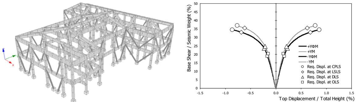
Figure 3. Finite element model (*left*) and capacity curves (*right*) of the retrofitted sample framed building.
