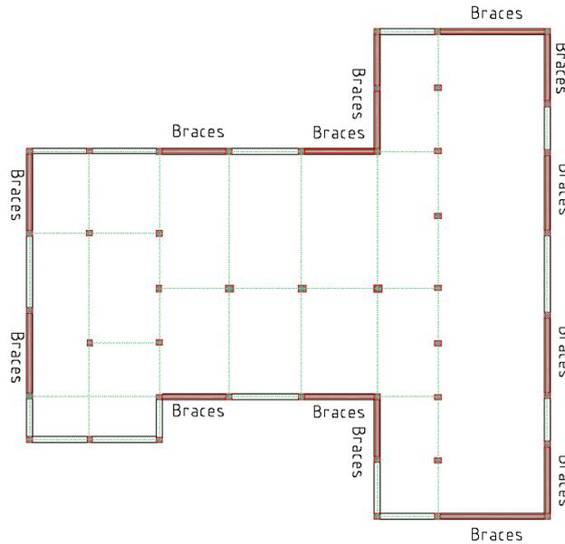
Figure 2. Layout of the dissipative braces along the perimeter of the T-shaped building block.
