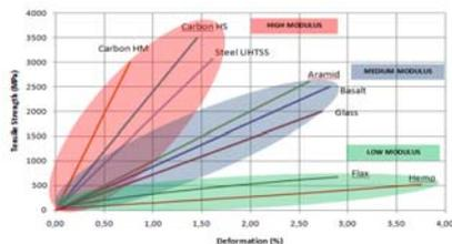
Figure 2. Comparison of different retrofit systems for strengthening structures.
