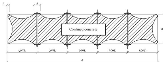
Figure 4. Confinement of rectangular section using FRP sheets and transversal steel bars.
