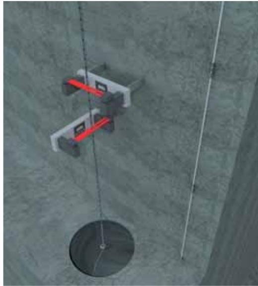
Figure 8. View of the pendulum (left) and Michelson optic fibre sensor (right)
