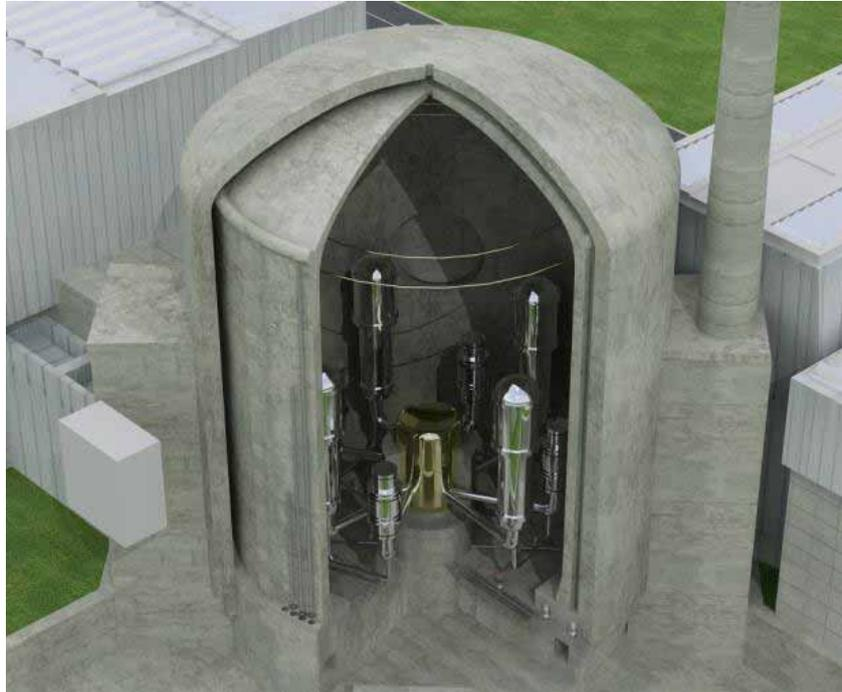
Figure 1. Double wall containment – cutaway
