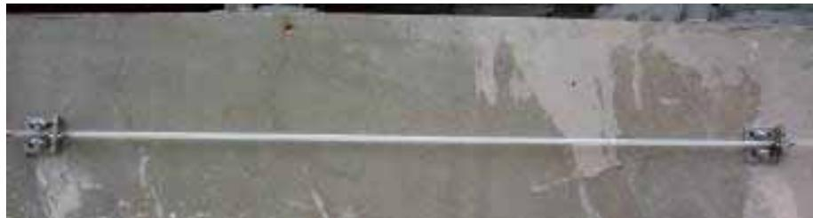
Figure 7. View of a long base optic fibre sensor
