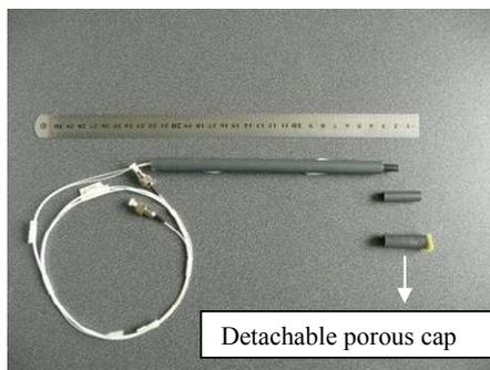
Figure 7. FOS-RH probe with FBG based humidity and temperature sensors
