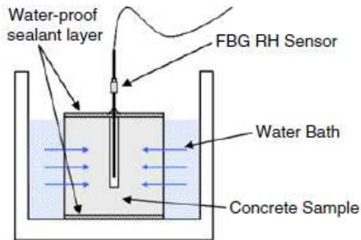
Figure 5. The fibre optic RH probe inserted centrally to monitor ingress of water
