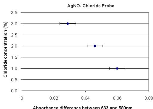
Figure 14. Calibration of sol-gel based chloride probe using silver nitrate as indicator
