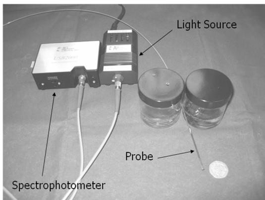
Figure 10. Fibre optic pH sensor set-up
