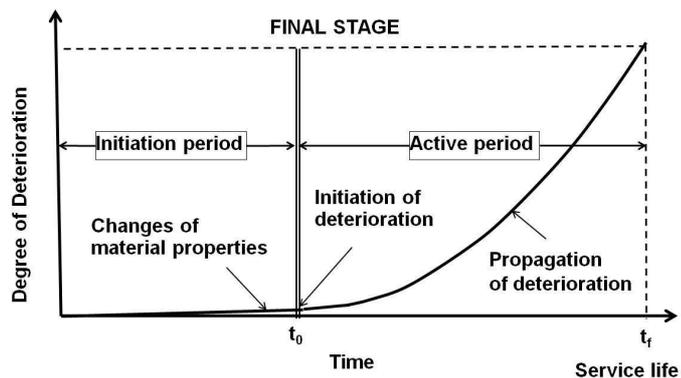
Figure 2. Usefulness of continuous monitoring of structures
