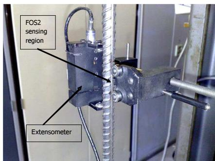
Figure 3. Steel bar with FBG sensor attached along with extensometer
