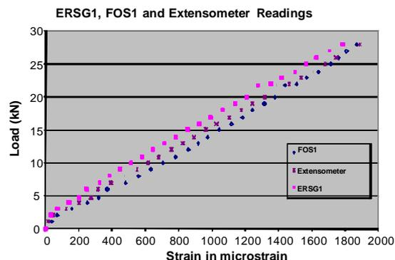
Figure 4. Comparison of results from FOS1(FBG), ERSG1 and extensometer showing change in strain ( $\mu\epsilon$ ) as a function of load (kN)
