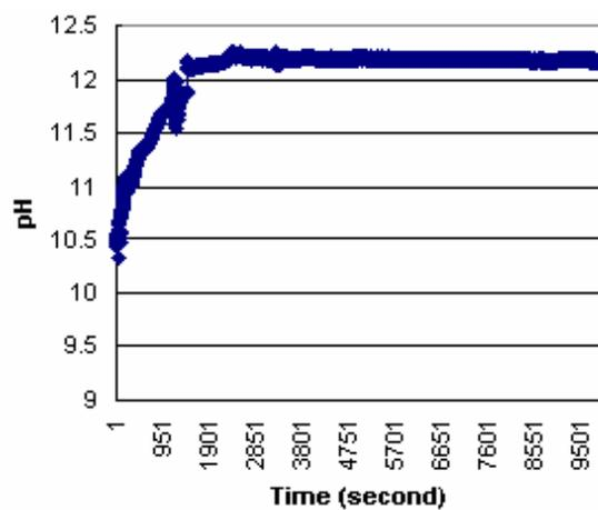
Figure 11. pH change with time in mortar sample using sol-gel based pH probe
