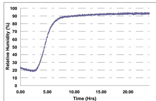
Figure 8. Change in RH with time monitored in concrete in a capillary rise test using Fibre optic RH probe
