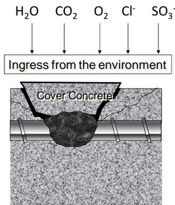
Figure 1. Environmental penetrations into concrete
