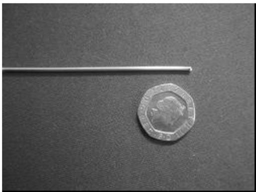
Figure 13. Sol-gel based chloride sensitive fibre optic probe
