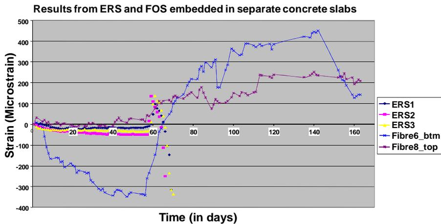
Figure 9. Strain measurements from ERSs and FBG sensors during accelerated corrosion test
