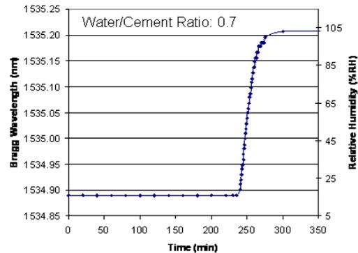
Figure 6. The change in Bragg wavelength due to ingress of water in concrete sample
