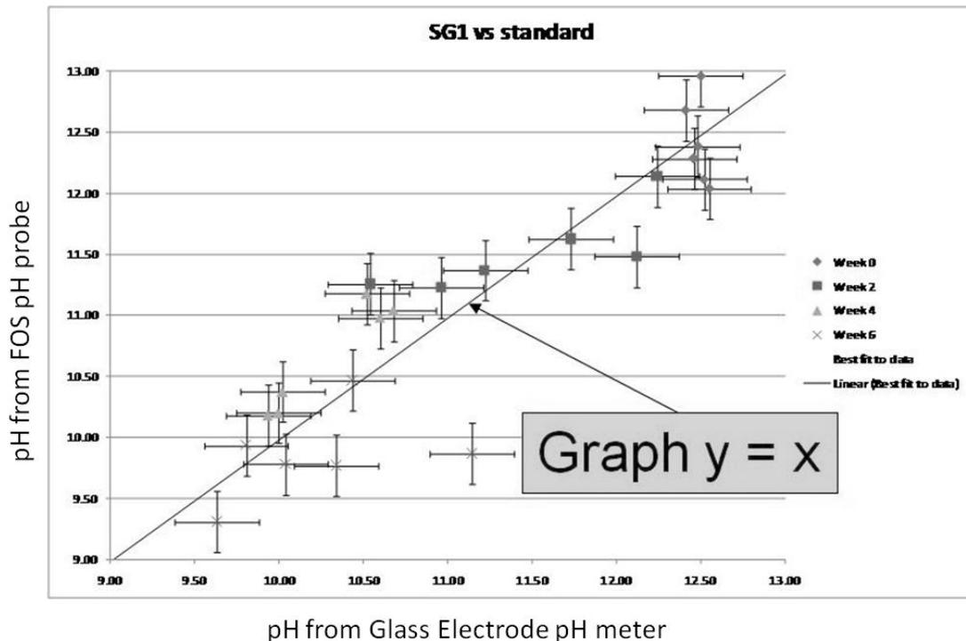
Figure 12. Comparison of fibre optic pH sensor with standard glass pH electrode for determining the effect of different degrees of carbonation on the pH of concrete.
