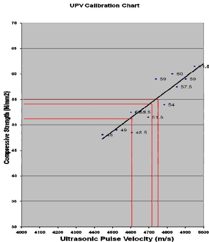
Figure 7. Typical UPV vs. compressive strength calibration chart.
