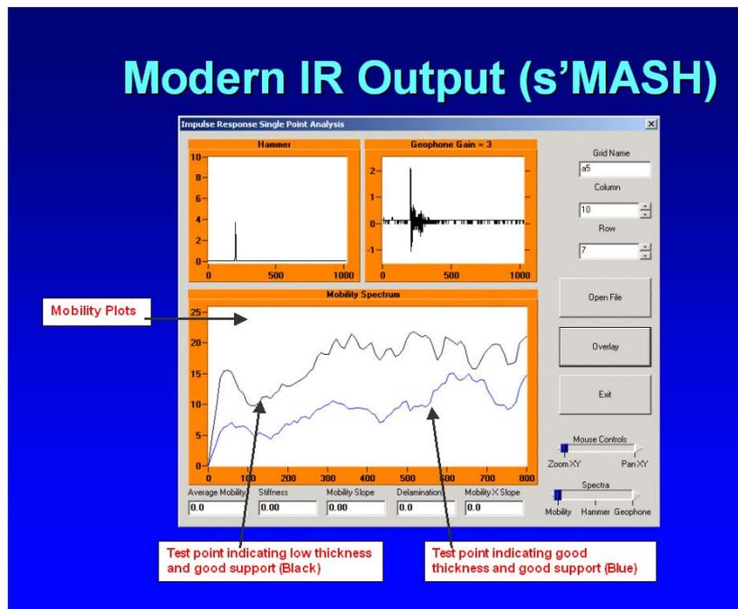
Figure 1. Typical response output of Impulse Response test.
