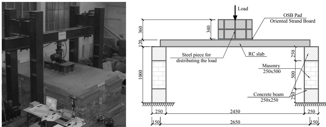
Figure 2. General view and a transversal cross section through the test setup.
