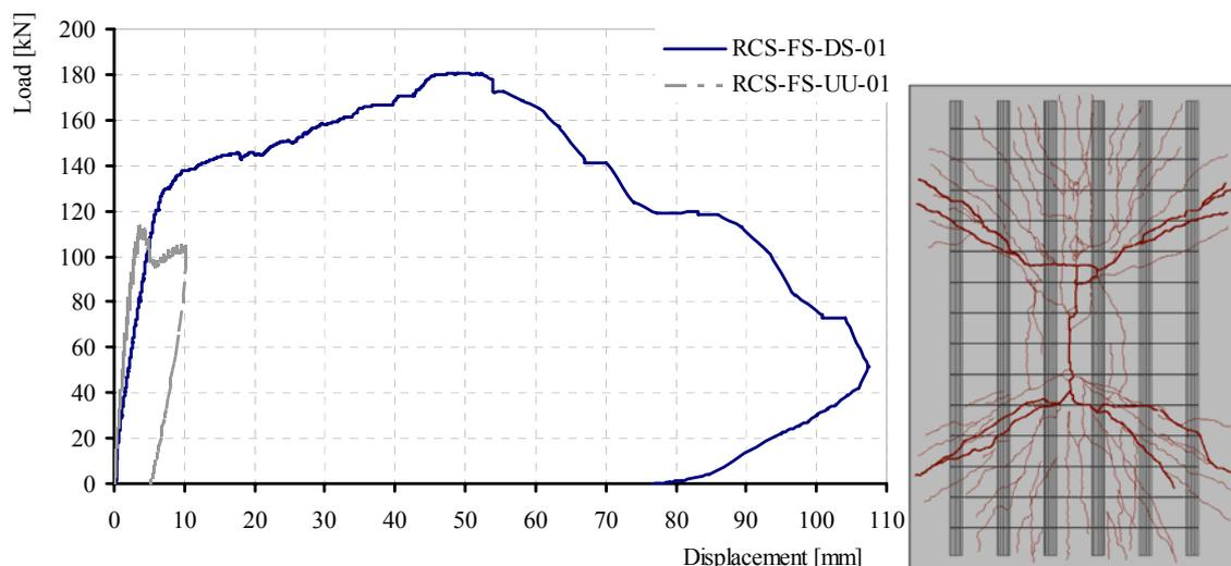
Figure 4. Load-displacement diagrams for RCS-FS-UU-01 and RCS-FS-DS-01 and crack pattern for RCS-FS-DS-01 slab.
