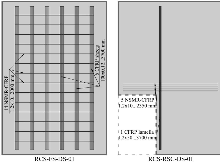
Figure 3. Retrofitting solutions for the two slabs.
