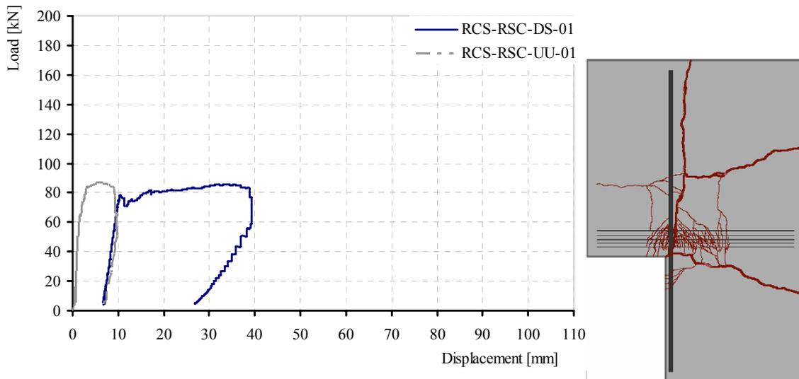
Figure 5. Load-displacement diagrams for RCS-RSC-UU-01 and RCS-RSC-DS-01 and crack pattern for RCS-RSC-DS-01 slab.
