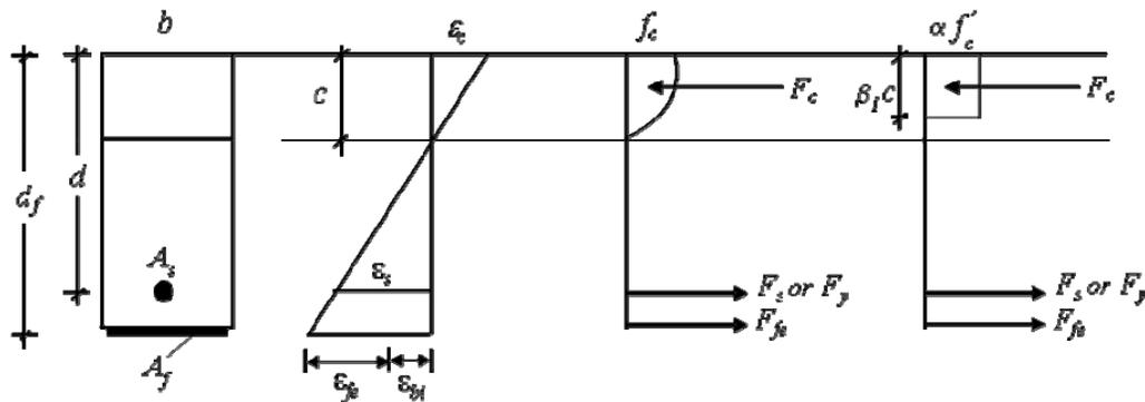
Figure 1: Internal strain and stress distribution at ultimate limit state [ACI 440.2R-08 2008]
