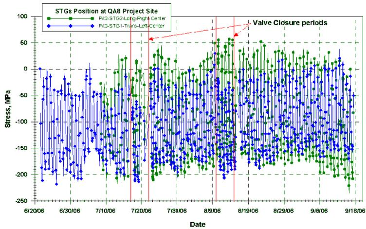
Figure 14. Stresses on buried pipeline in pit #2.
