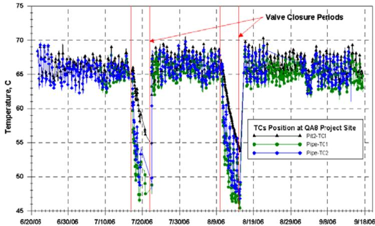
Figure 8. Surface temperatures on buried and exposed pipeline.
