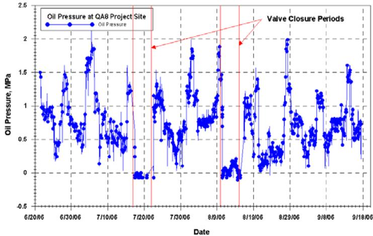
Figure 9. Oil pressure in the pipeline.
