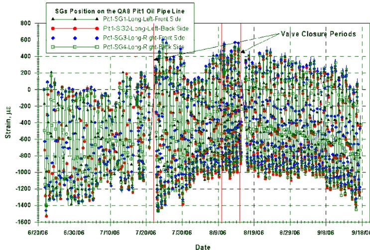
Figure 11. Strain in buried pipeline in pit #1.
