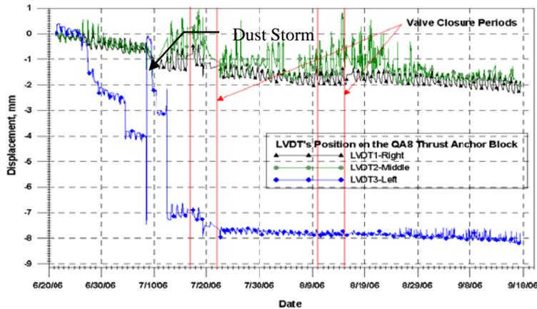
Figure 15. Vertical movement of anchor block.
