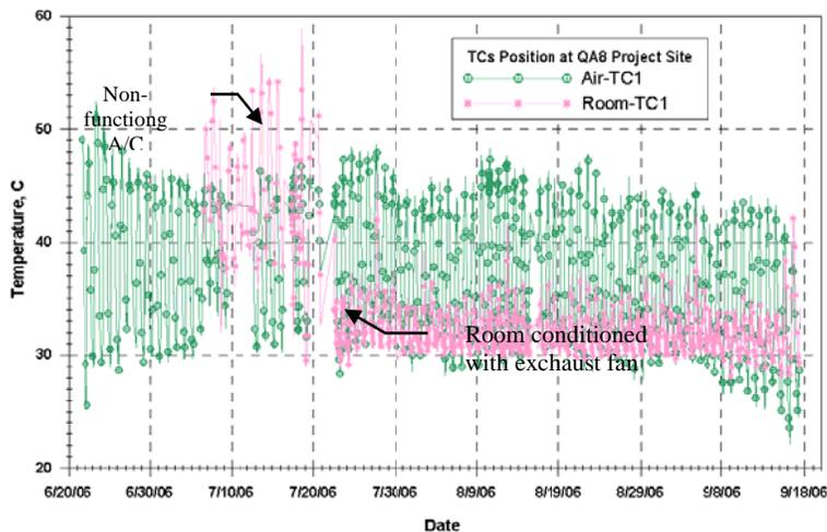
Figure 7. Ambient and mobile-lab temperatures at the Abqaiq site.
