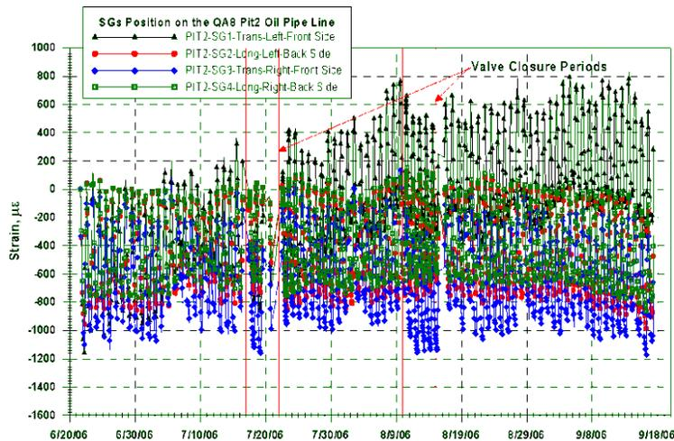
Figure 12. Time series plots for strain in buried pipeline in pit #2.
