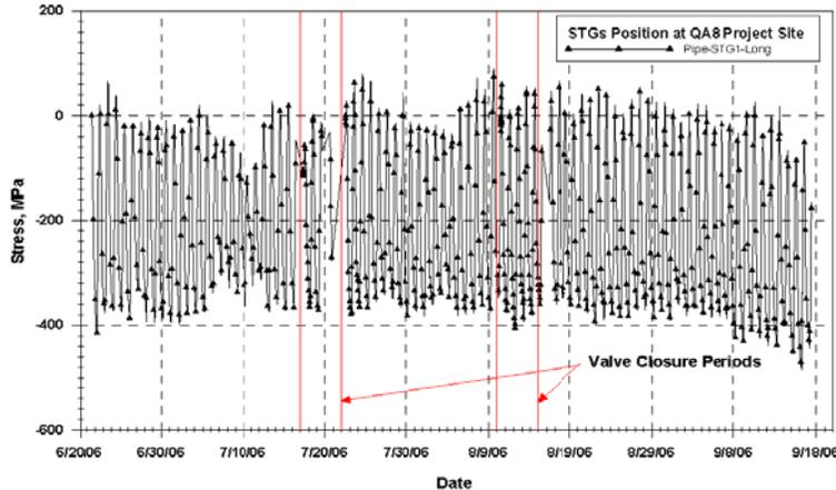
Figure 13. Stresses measured on exposed pipeline.
