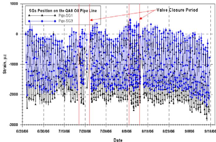
Figure 10. Strains on exposed oil pipeline.
