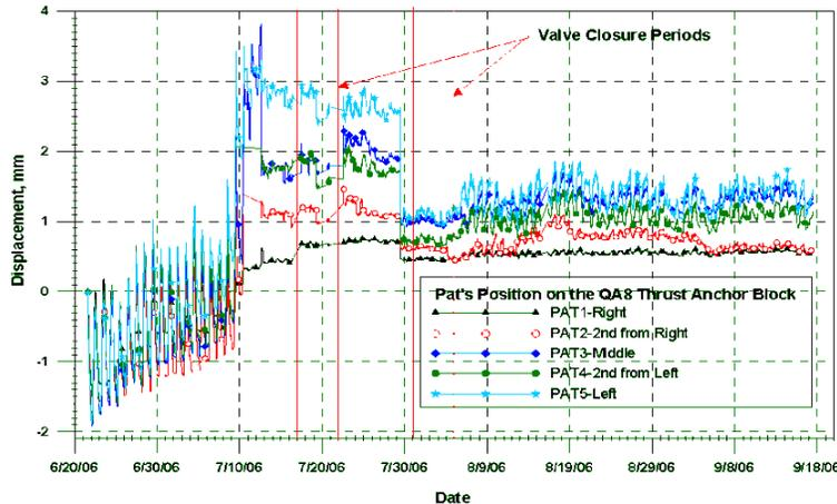
Figure 16. Horizontal displacement of thrust anchor block.
