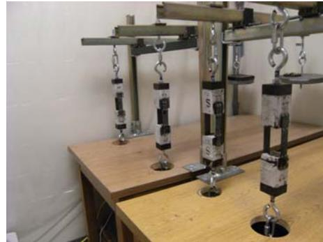
(b) Four creep specimens loaded
