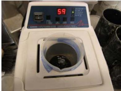
(a) Sonication of CNTs in epoxy resin
