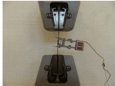
(b) Single shear CFRP-CFRP interface
