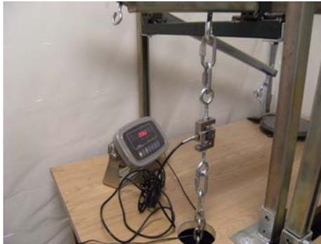
(a) Load cell attached to determine creep load
