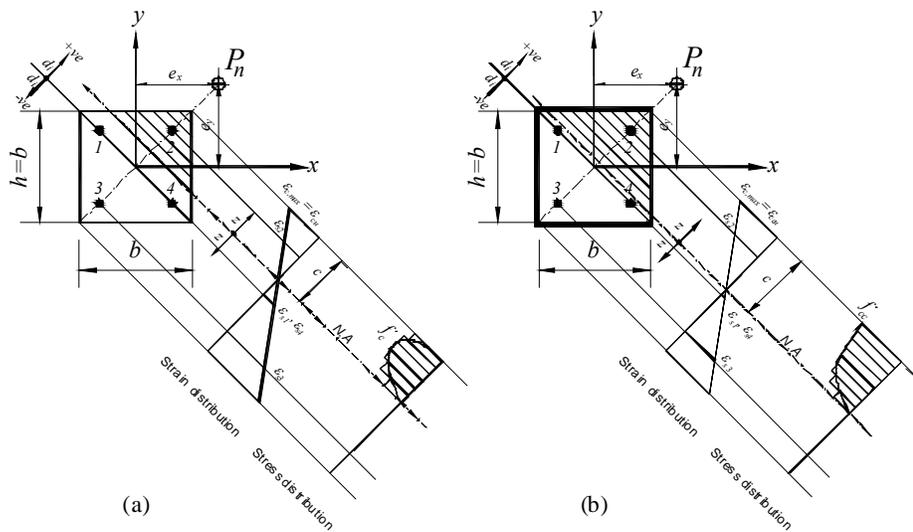
Figure 6. Distribution of strains and stresses for a symmetric square cross-section under biaxial eccentric loading; (a) unconfined section, (b) CFRP-confined section
