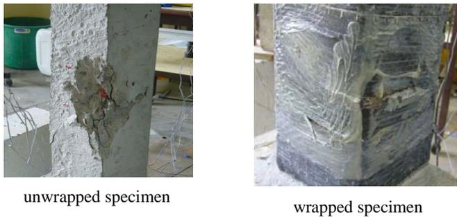
Figure 3. Failure modes under biaxial loading
