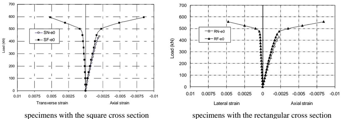
Figure 4. Load-strain relationships of the concentrically loaded columns
