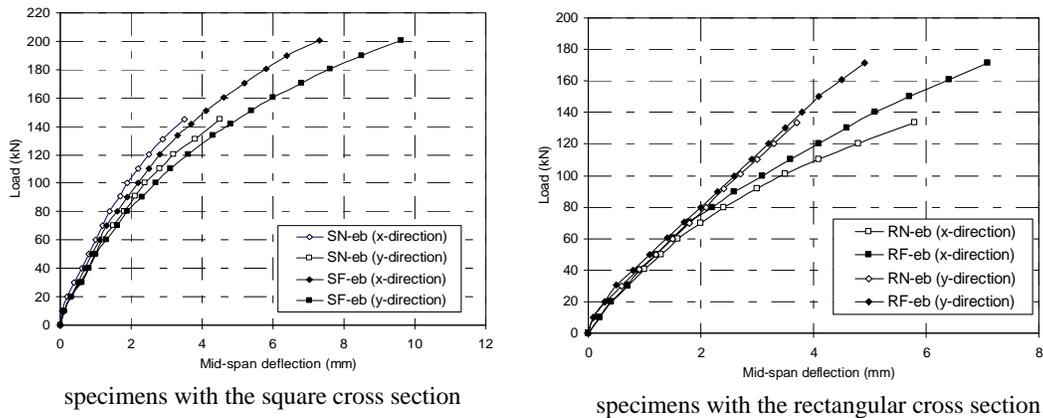
Figure 5. Load-lateral deflection relationships of the columns tested under biaxial eccentric loading
