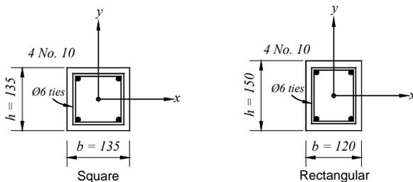
Figure 1. Cross sections shapes
