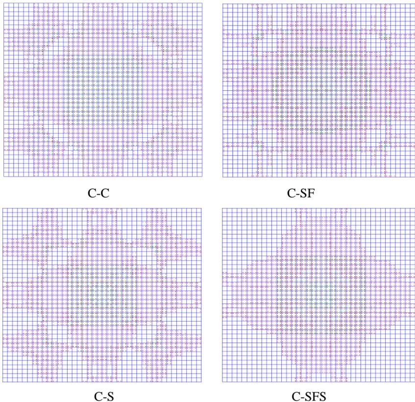
Fig. 3 Crack distribution for various overlays
