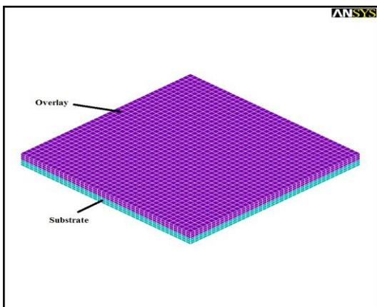
Fig. 1 Modeling of bonded concrete overlay in ANSYS
