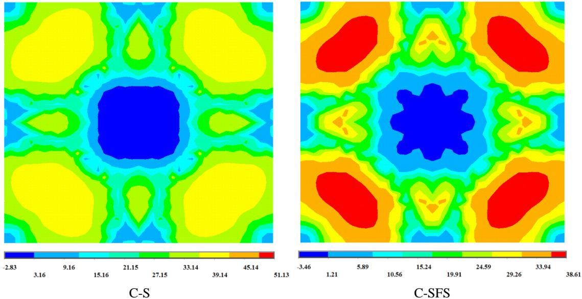
Fig. 3 Principal stress distribution in two different overlays
