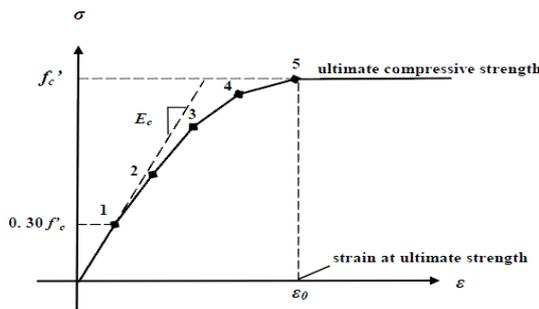
Fig. 2 Simplified compressive uniaxial stress-strain curve for concrete
