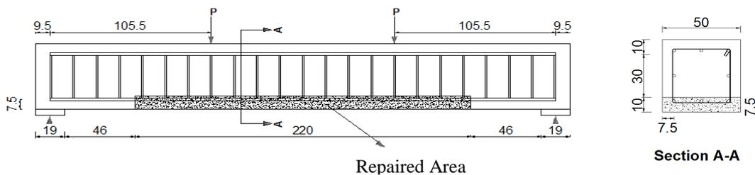
Fig. 2 Details of specimen, reinforcement and the location of repair
