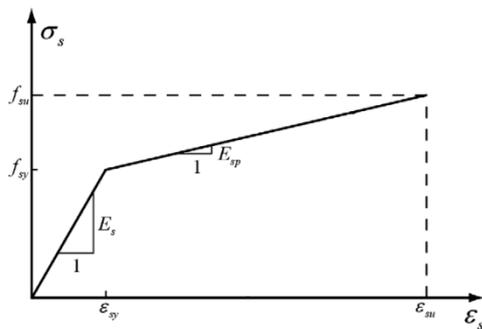
Fig. 4 Idealization of steel stress–strain behavior
