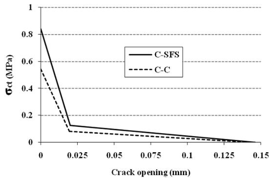
Fig. 5 Tension softening model for simulation of debonding behavior of repair system
