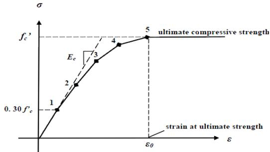
Fig. 3 Simplified compressive uniaxial stress-strain curve for concrete
