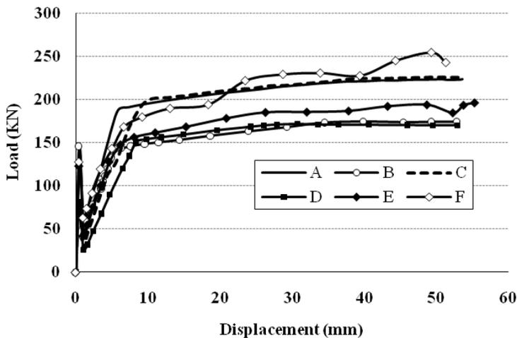
Fig. 7 Load-deflection curves for investigated beams
