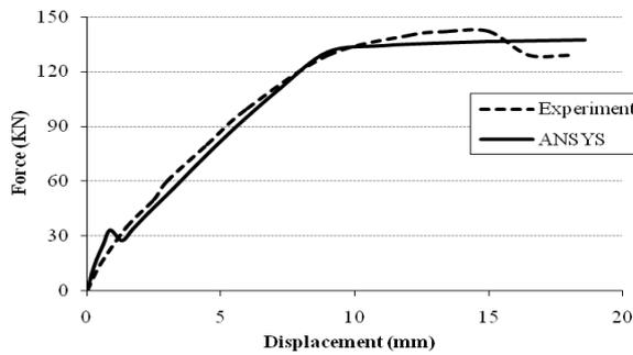
Fig. 6 Comparison between experimental results and numerical simulation for “FCB1R-O”
