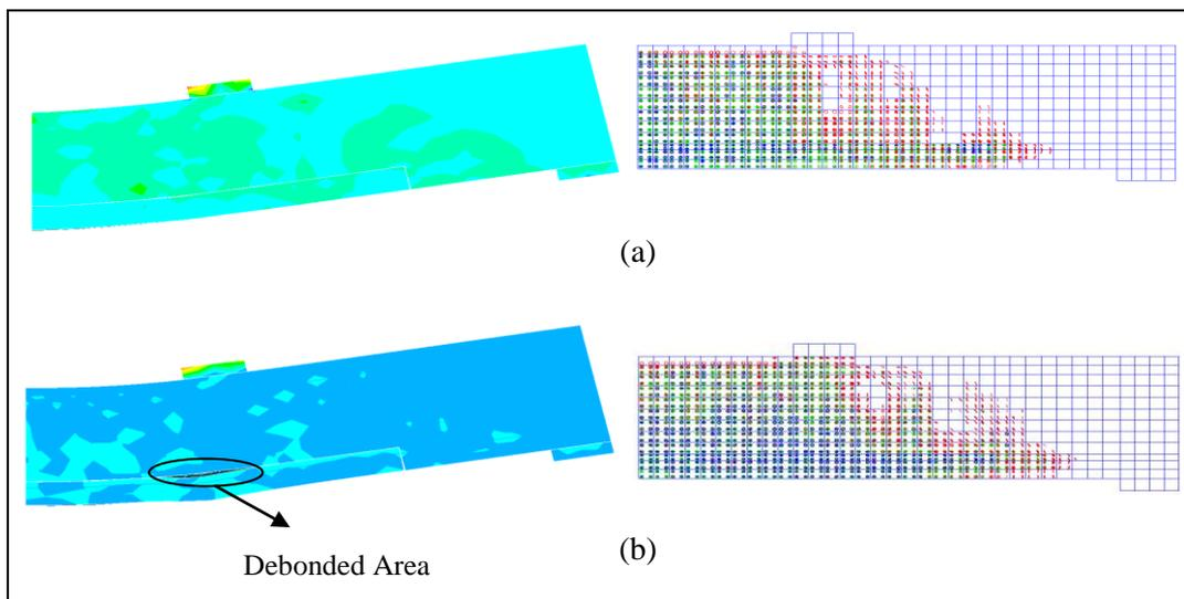
Fig. 8 Principal stress and crack distributions in repaired beams with repair mix designs C-C (a) and C-SFS (b)
