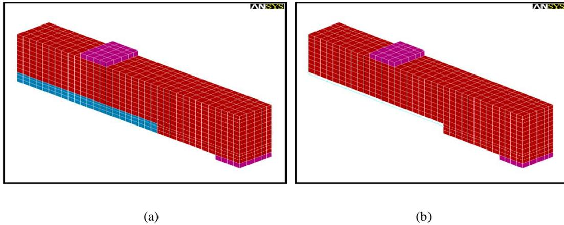
Fig. 1 Modeling of quarter part of (a) repaired and (b) deteriorated reinforced concrete beams
