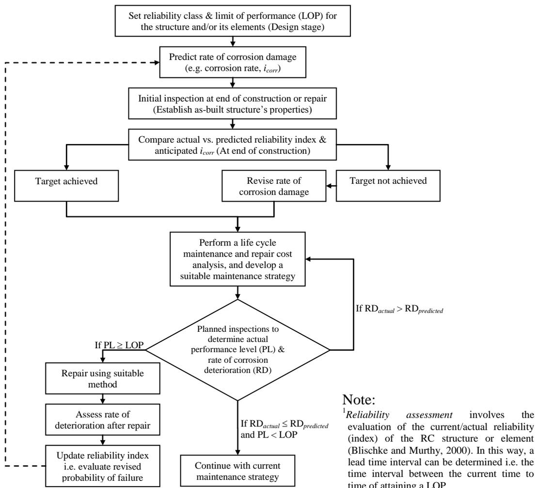
Figure 2: Example of a pro-active risk-based maintenance and repair programme
