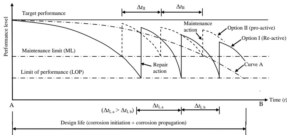
Figure 1: Maintenance and repair strategies for RC structures (modified from (Bijen, 1989))
