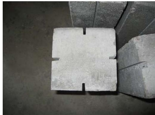
Figure 3b. four slits each of dimensions 18 x 5 mm for specimens strengthened by four exterior CFRP slotted strips.
