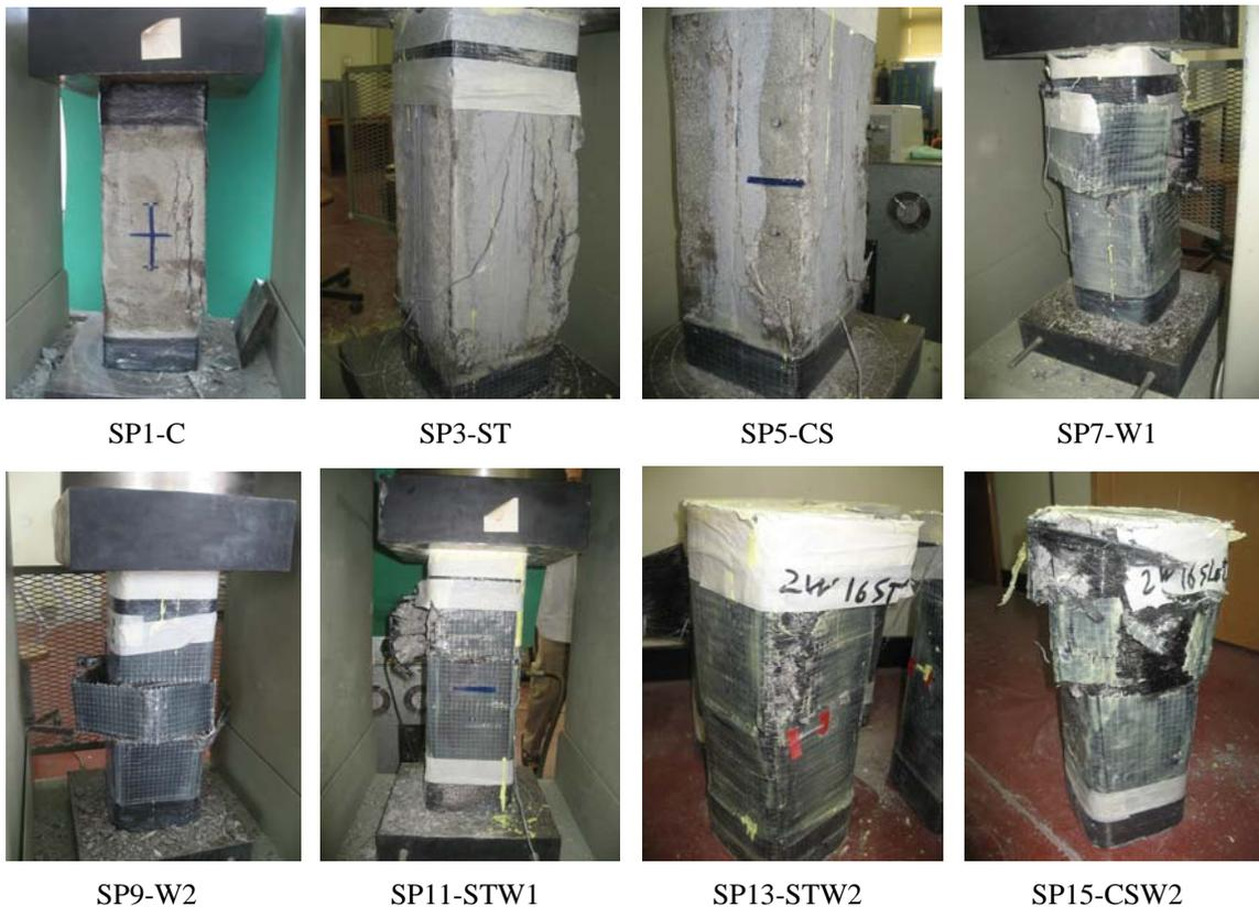
Figure 4. Failure of different tested specimens
