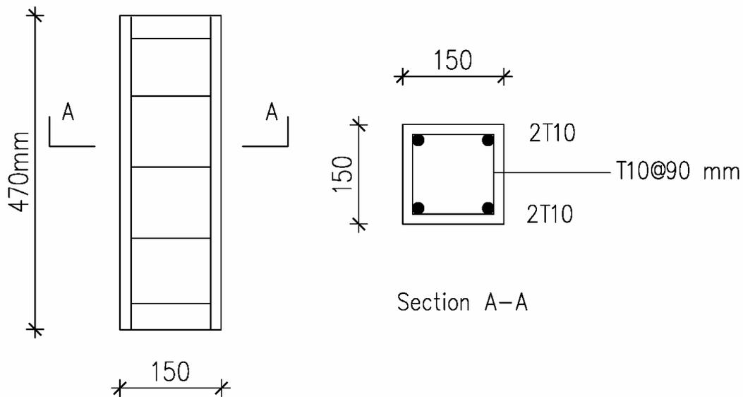
Figure 2. Columns dimensions and reinforcement.
