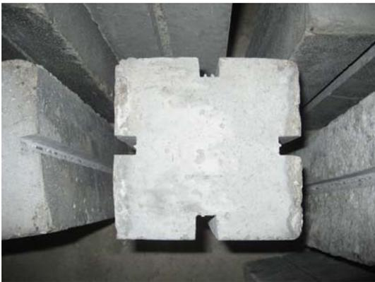
Figure 3a. four slits each of dimensions 18 x 18 mm for specimens strengthened by four exterior steel bars 12 mm diameter.
