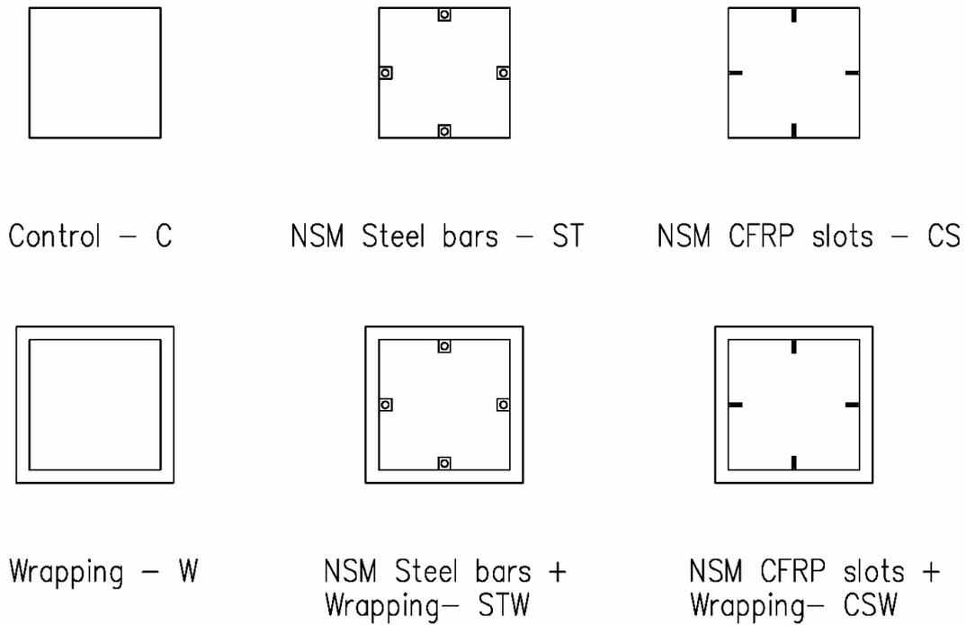
Figure 1. Different types of columns strengthening.
