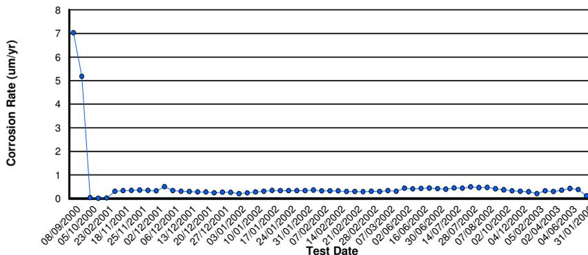
Figure 2: Corrosion Penetration Rate of SACI in Clifton Bridge
