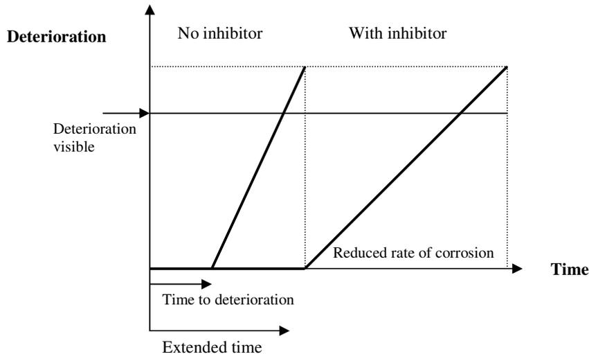
Figure 1: Concept of Extending of the service life of RC structures with corrosion inhibitor, Laamenen & Byfors (1996)
